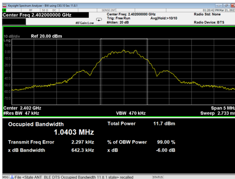
27 Occupied Bandwidth, Low Channel, GMSK 1MB
