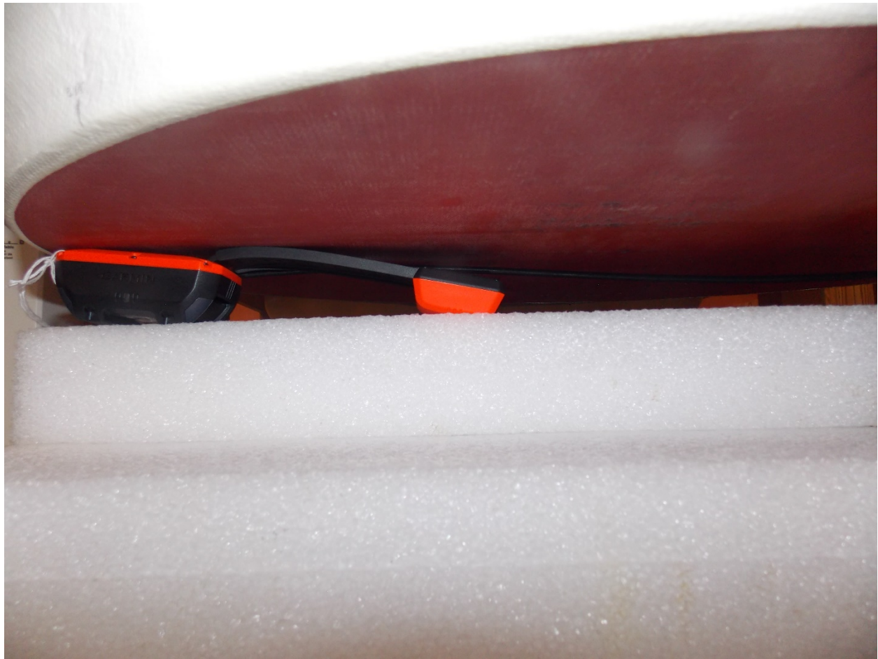
Test Position VHF Back 0 mm Gap
