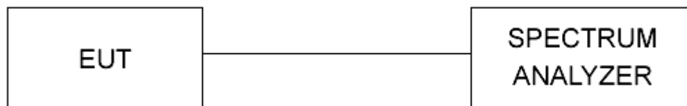
Figure 1 - Bandwidth Measurements Test Setup
