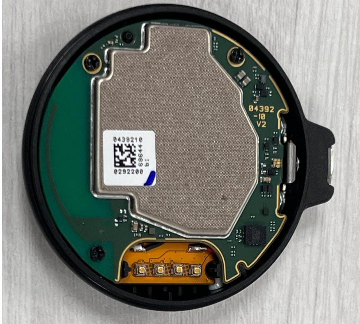
Photograph 6-1 : Front side view of the main board, shields in place
