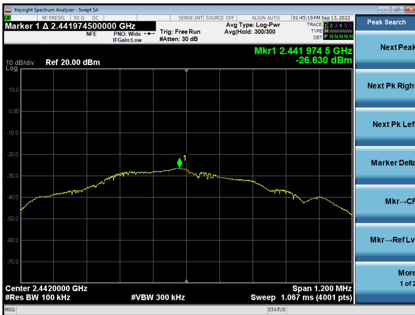
Figure Tr17.5: Partially corrected power spectral density data for ANT, 2442 MHz
