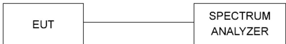
Figure 1 - Bandwidth Measurements Test Setup
