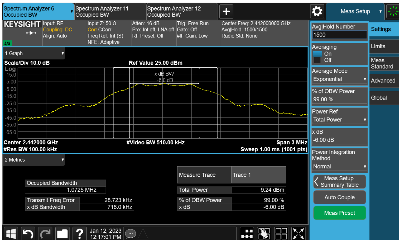
Figure TR8.3: Spectral data for BLE 1 Mbps on the Mid frequency.
