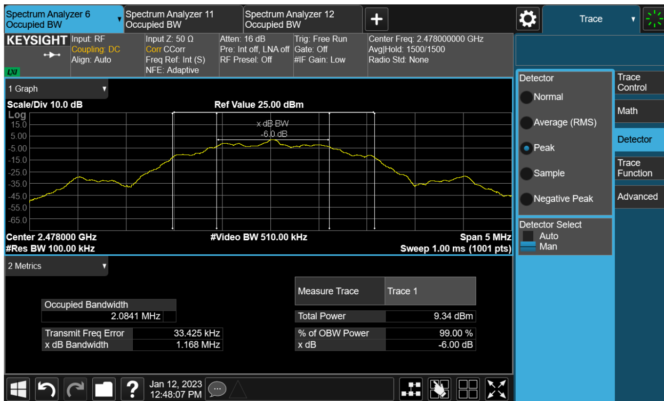
Figure TR8.7: Spectral data for BLE 2 Mbps on the High frequency.
