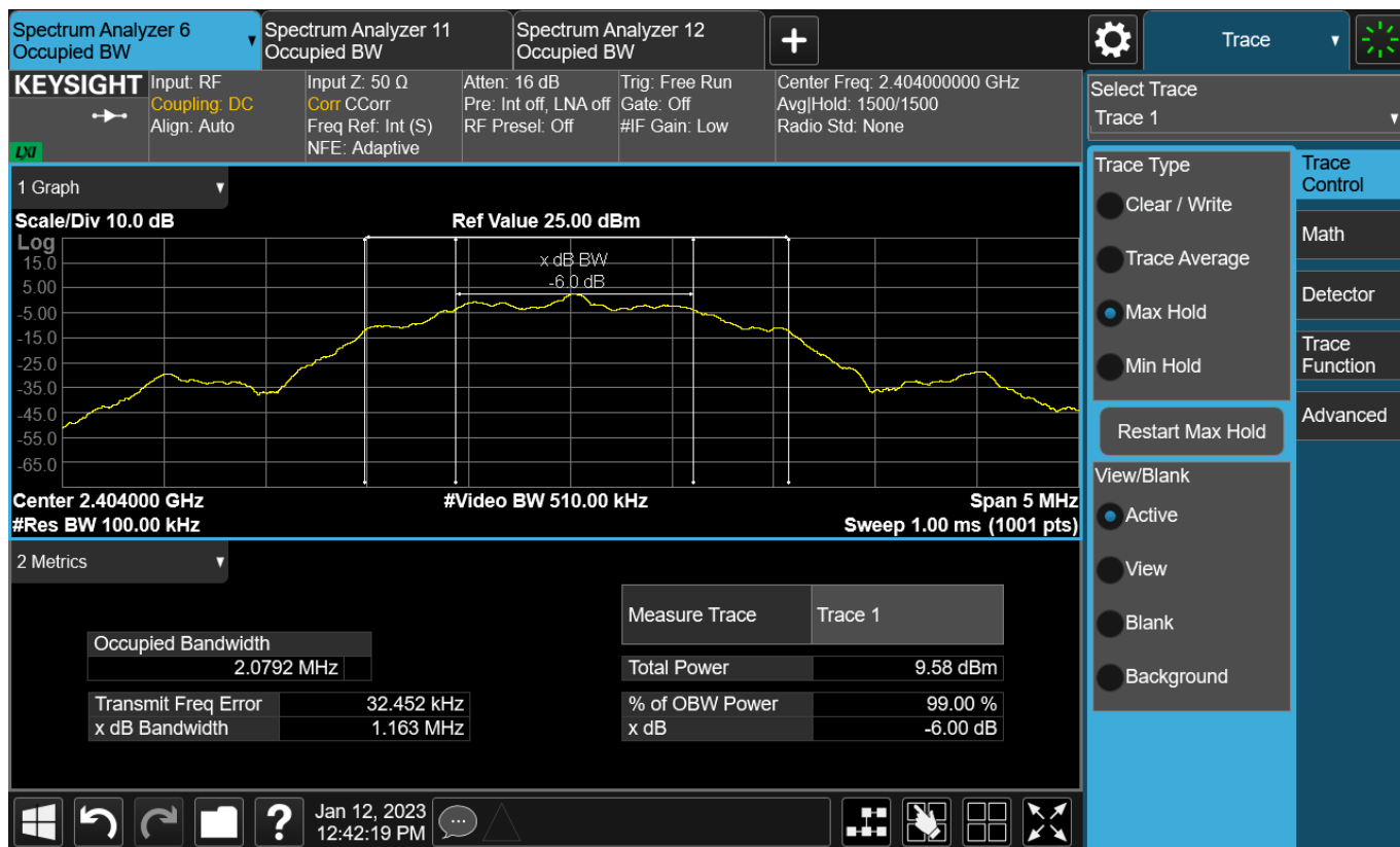
Figure TR8.5: Spectral data for BLE 2 Mbps on the Low frequency.
