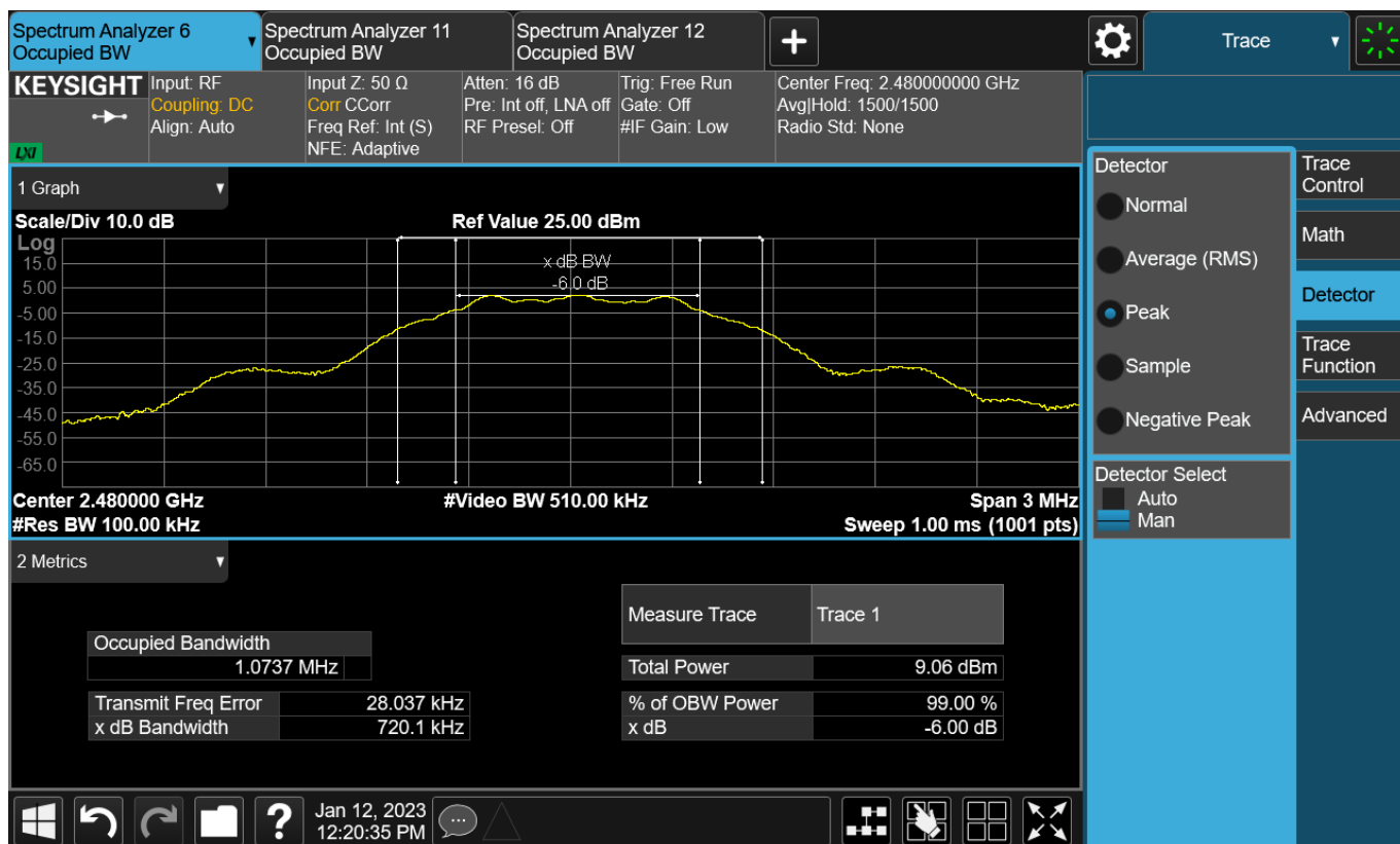
Figure TR8.4: Spectral data for BLE 1 Mbps on the High frequency.
