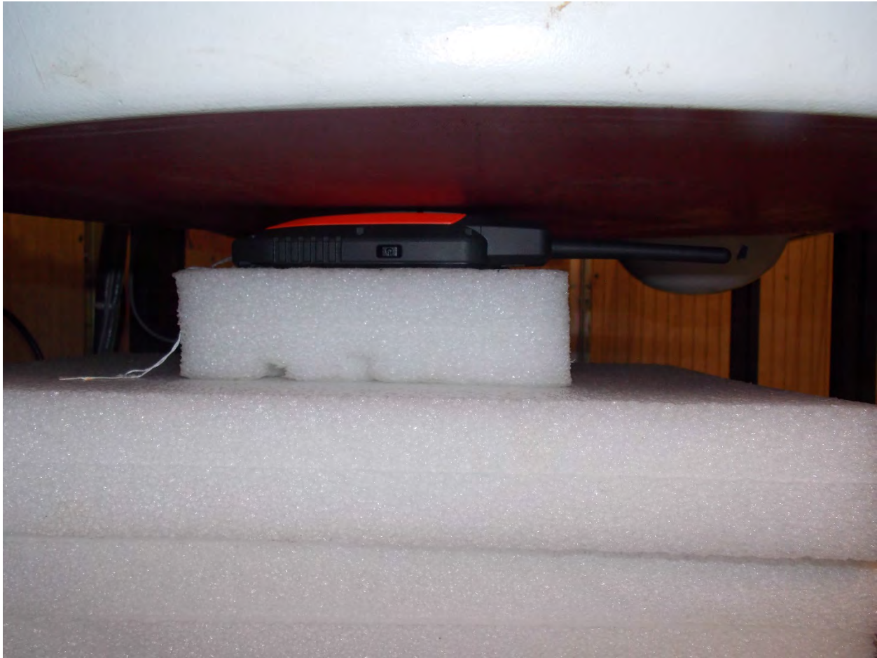
Test Position Back Short Antenna 0 mm Gap
