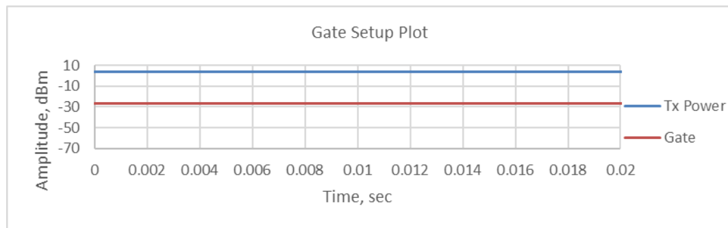
Figure TR02.2: Gate setting diagram for ANT Radio, 2440 MHz
