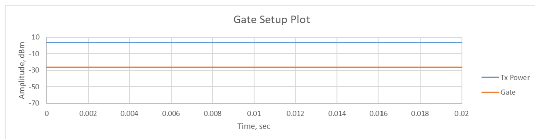
Figure TR02.1: Gate setting diagram for BLE Radio, 1 Mbps modulation, 2440 MHz
