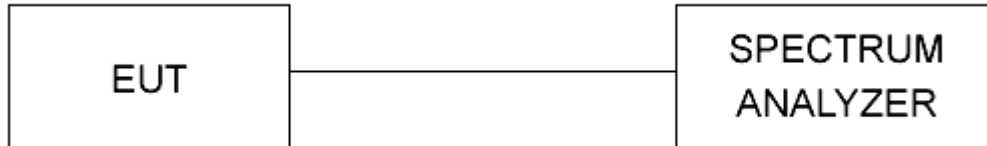
Figure 1 - Bandwidth Measurements Test Setup
