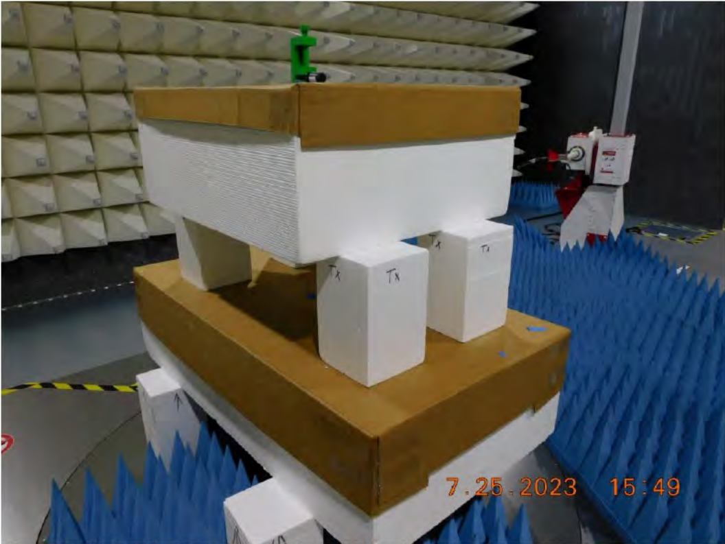
Figure RE01.4: EUT test setup, side view (X orientation)
