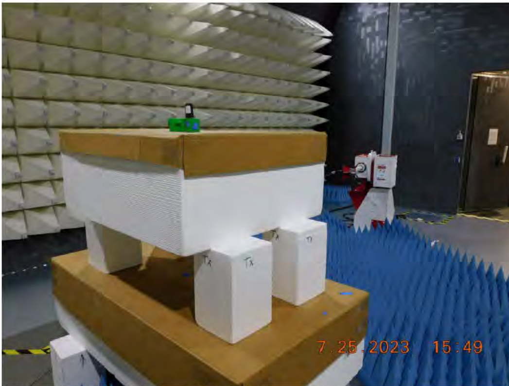
Figure RE08.4: EUT test setup, Z orientation
