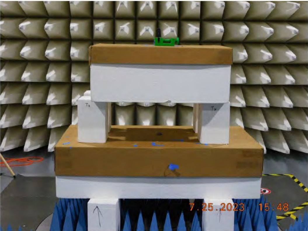
Figure RE05.2: EUT test setup, front view
