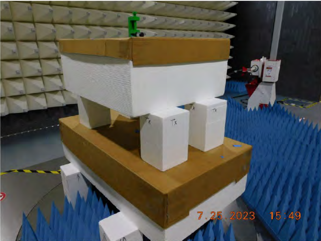
Figure RE08.2: EUT test setup, X orientation
