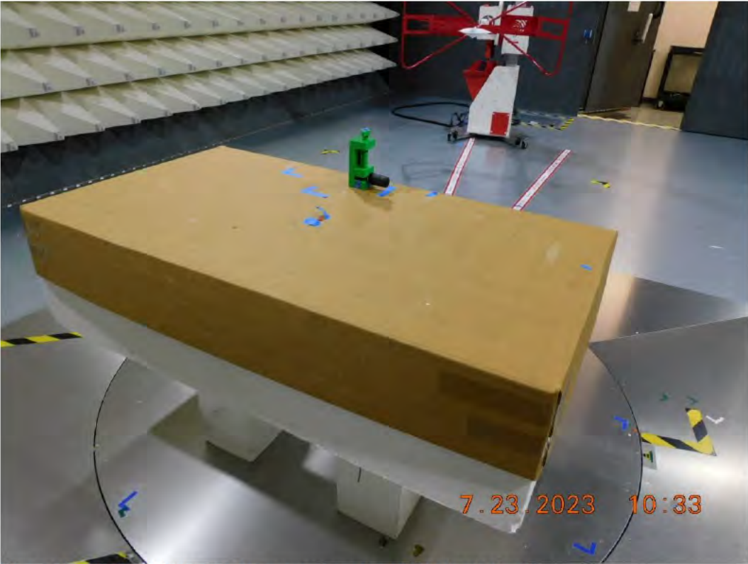
Figure RE07.5: EUT test setup, reverse view (X Orientation)
