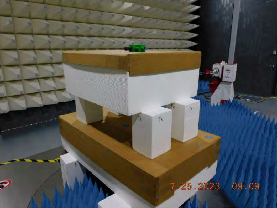
Figure RE08.3: EUT test setup, Y orientation
