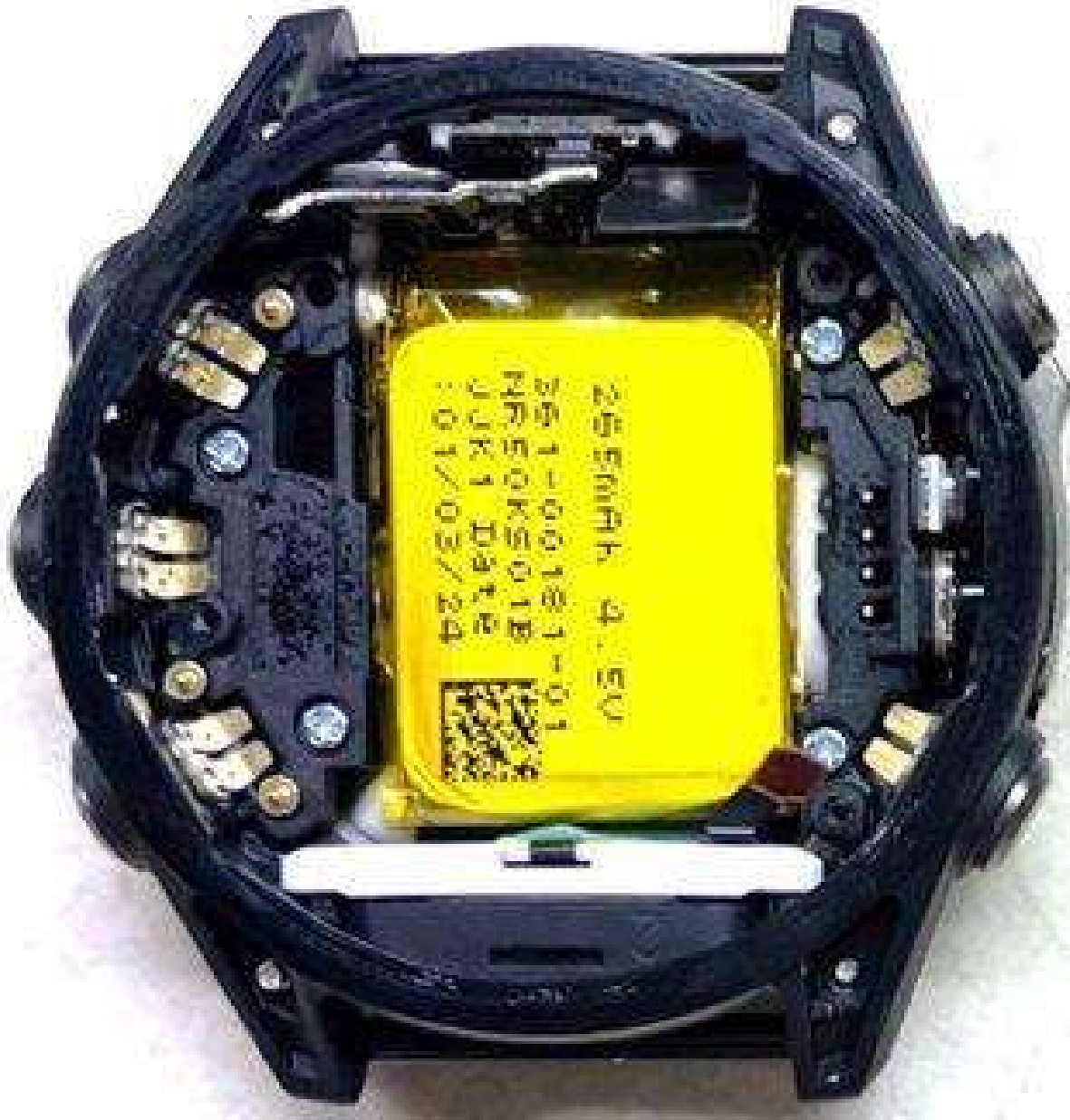
Figure E14.2 – Internal – DUT, Main PCB Removed
