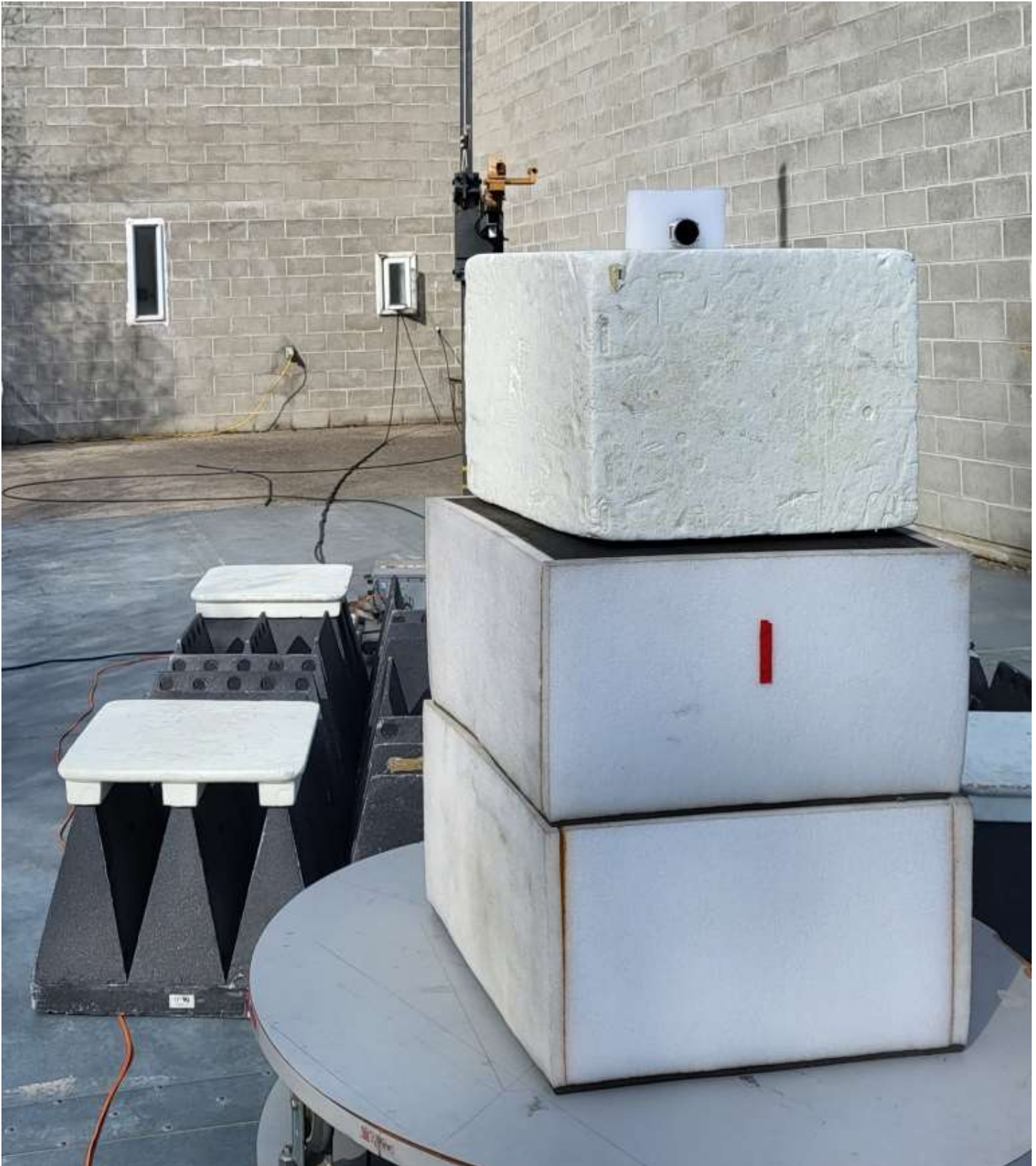
Figure E15.6 – Setup, Radiated Tx Measurements 18 – 26GHz
