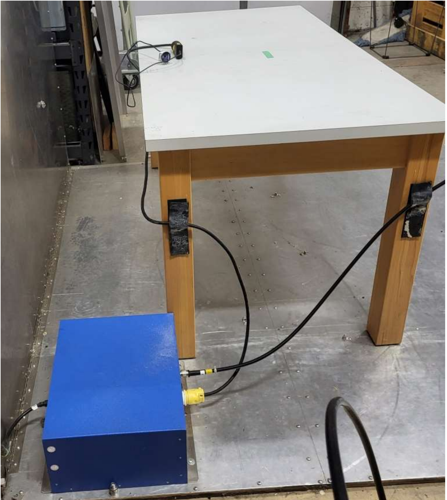
Figure E15.7 – Setup, Line Conducted Measurements
