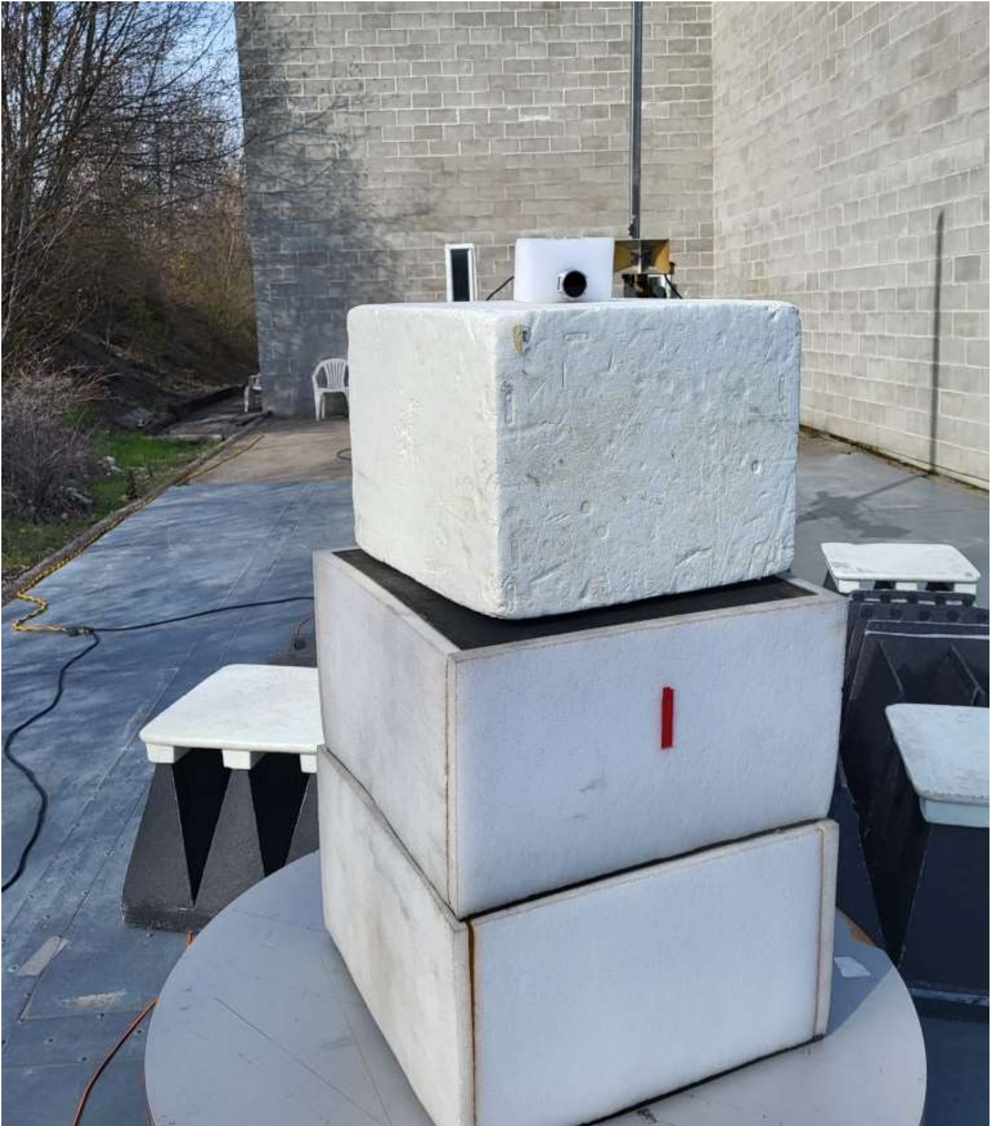
Figure E15.5 – Setup, Radiated Tx Measurements 1 – 18GHz
