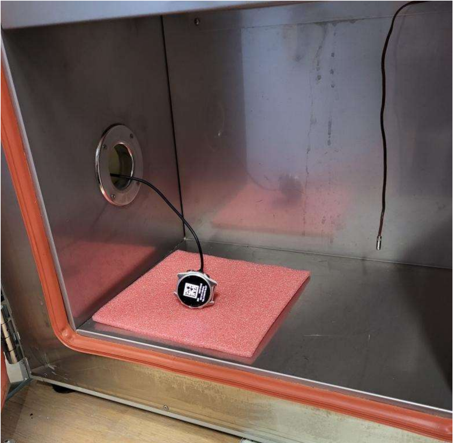
Figure E15.9 – Setup, Frequency Stability Measurements
