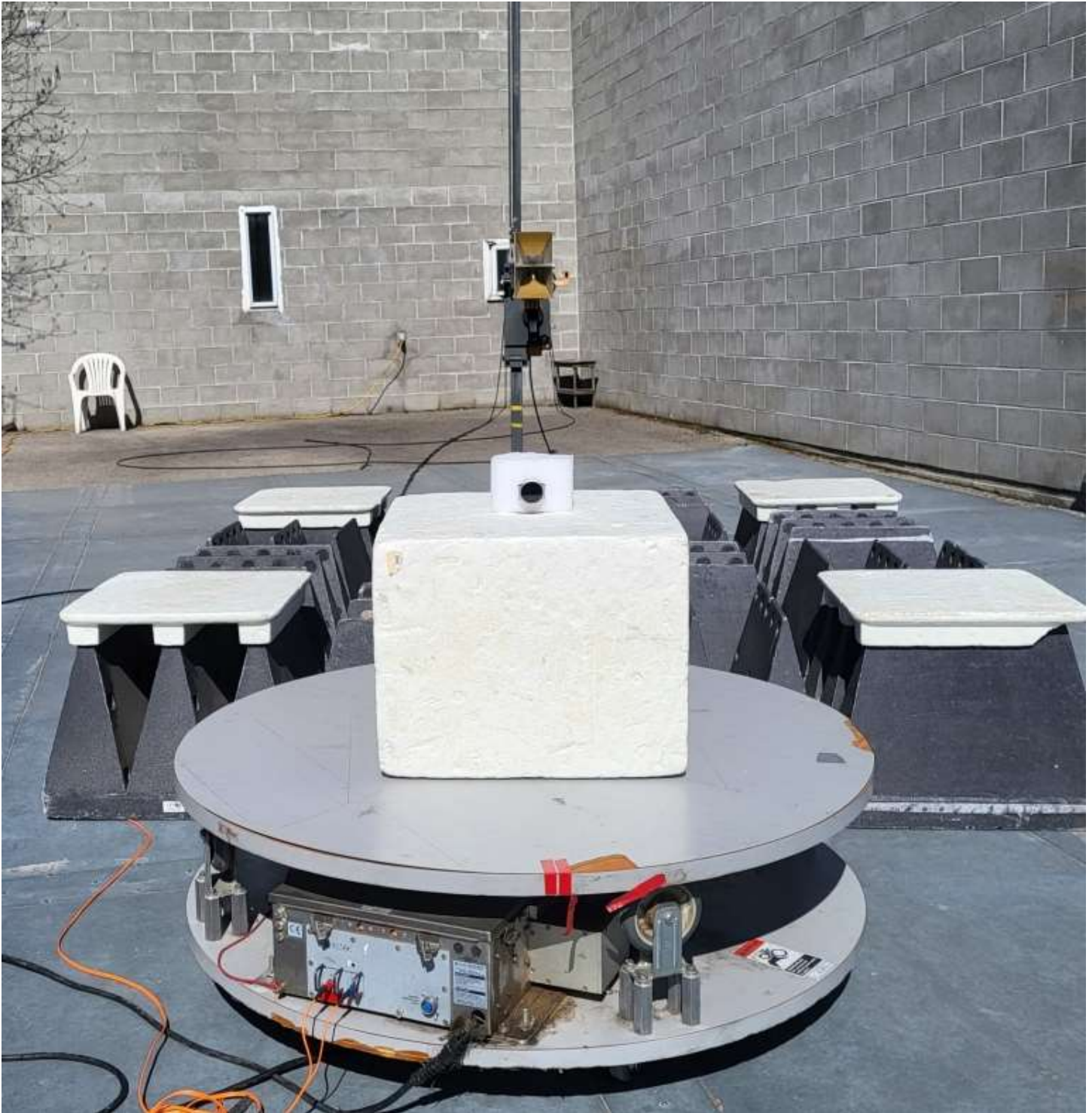
Figure E15.4 – Setup, Radiated Rx Measurements 1 – 18GHzHz
