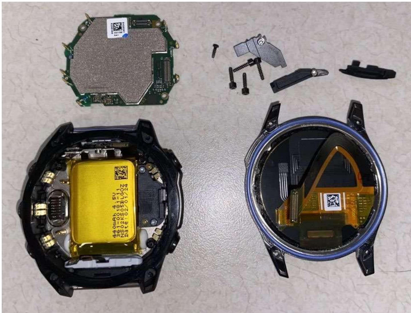
Figure E14.2 – Internal – DUT, Main PCB Removed
