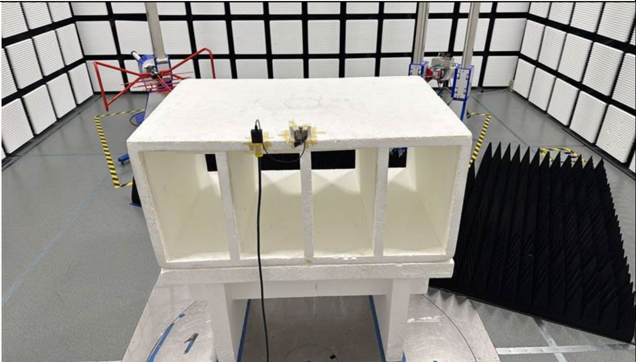
WWAN RADIATED MEASUREMENT SETUP ABOVE 1GHZ FRONT – LOW BAND
