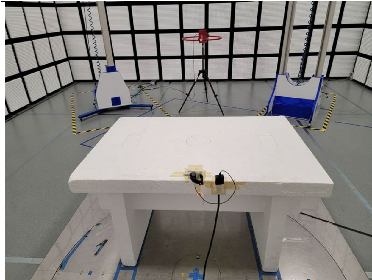
WWAN RADIATED MEASUREMENT SETUP BELOW 30MHZ FLAT.
