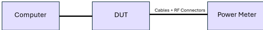
Figure 3-1 FTM Power Measurement Setup
