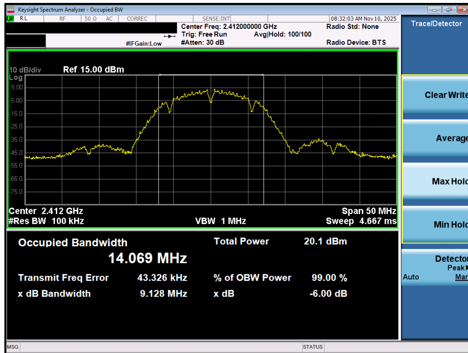
Plot 7-1. 6dB Bandwidth Plot (802.11b – Ch. 1)
