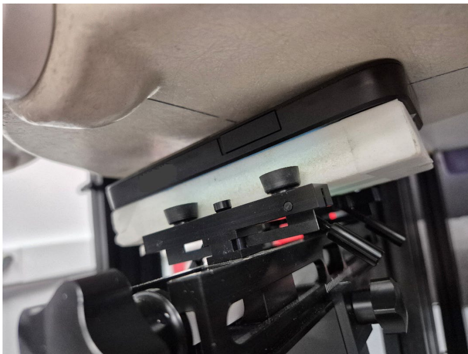
Figure 1 SAR Test Setup – Body/Extremity – Back Side 0mm
