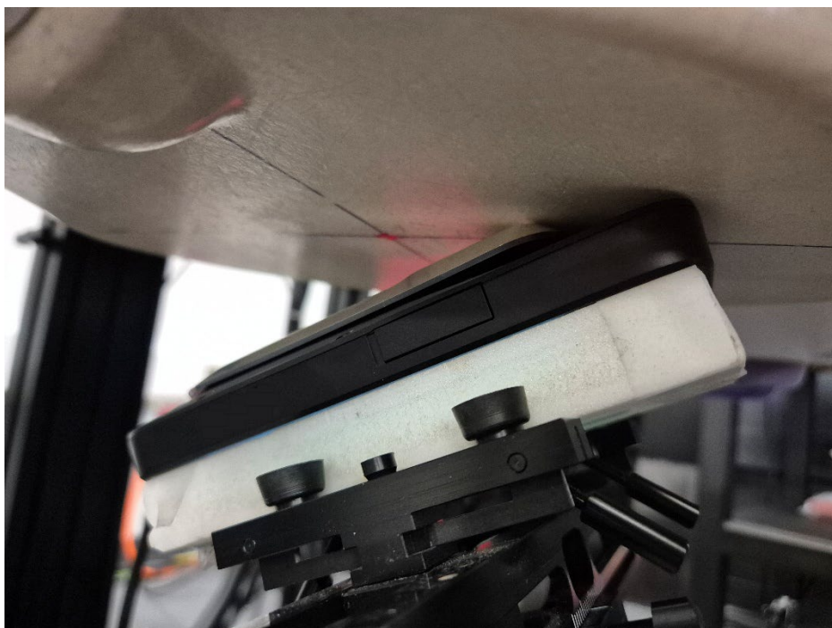
Figure 2 SAR Test Setup – Body/Extremity with Stand attached – Back Side 0mm
