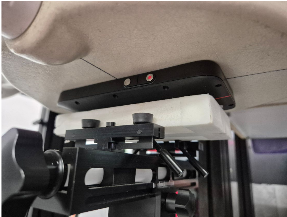
Figure 3 SAR Test Setup – Body/Extremity – Front Side 0mm
