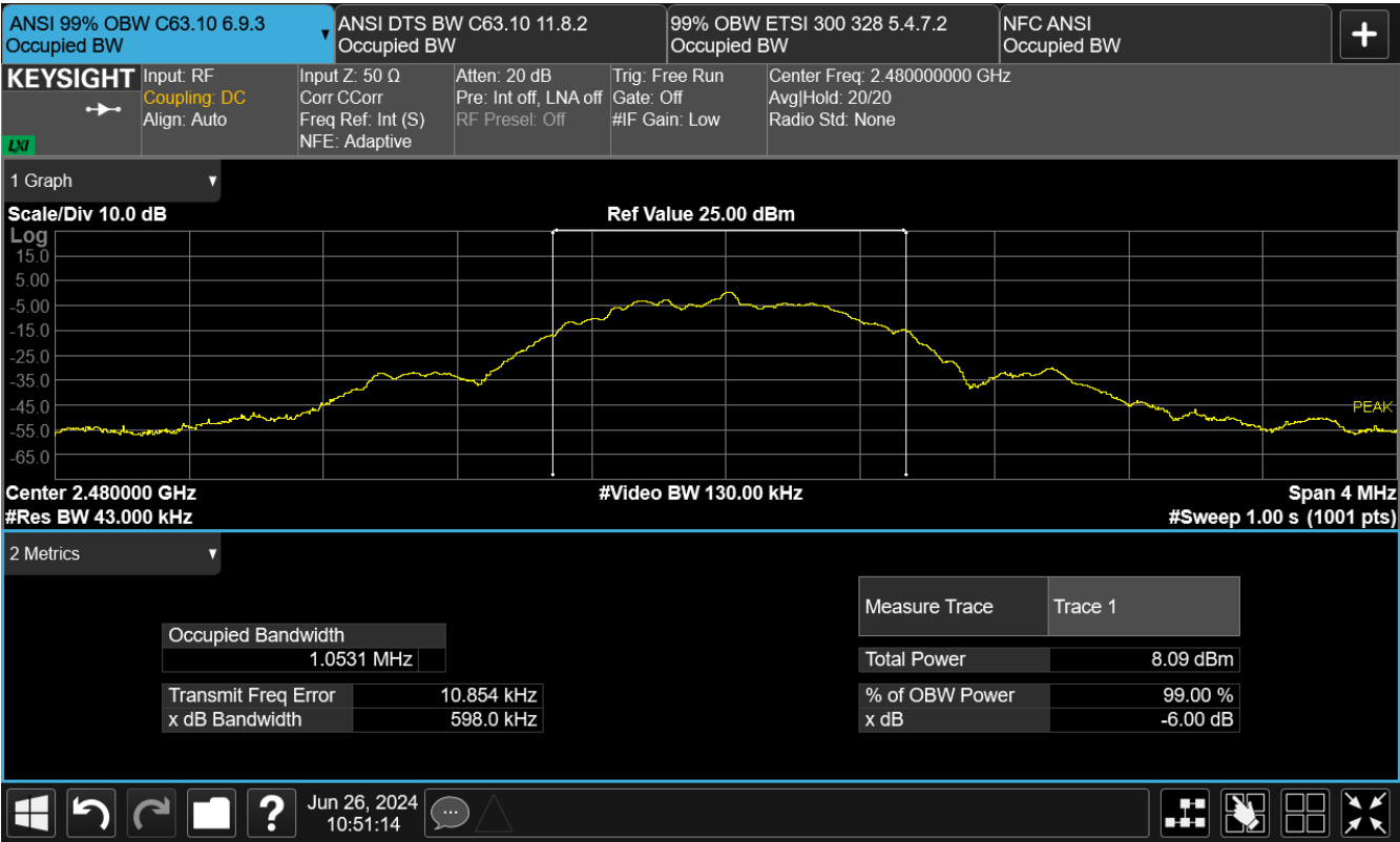
Figure TR10.2: Bandwidth data for BLE 1 Mbps at 2480 MHz
