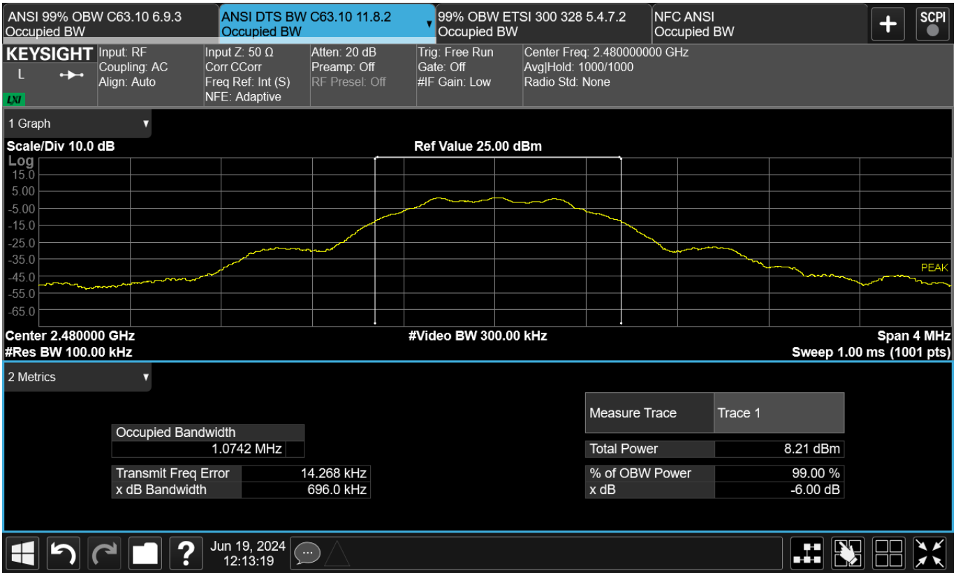
Figure TR06.2: Bandwidth data for BLE 1 Mbps at 2480 MHz
