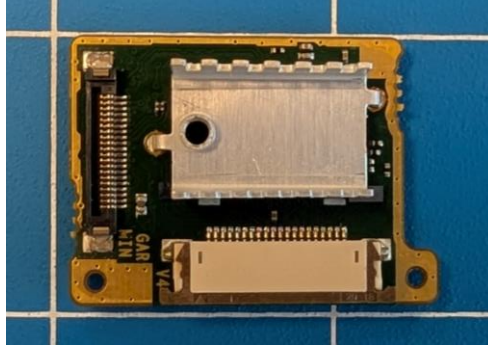
x04946 PCBA#3 Front without Absorber
