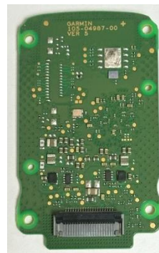
Photograph 07-4: Back side view of the radar board
