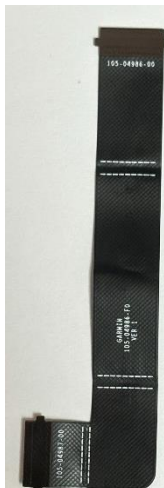
Photograph 07-5: Front side view of the radar FPC
