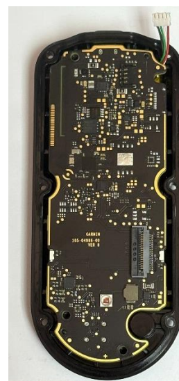
Photograph 07-8: Lower enclosure components – battery connector and screws removed
