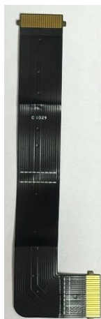
Photograph 07-6: Back side view of the radar FPC
