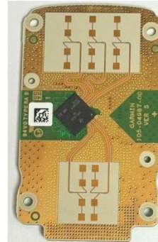
Photograph 07-3: Front side view of the radar board
