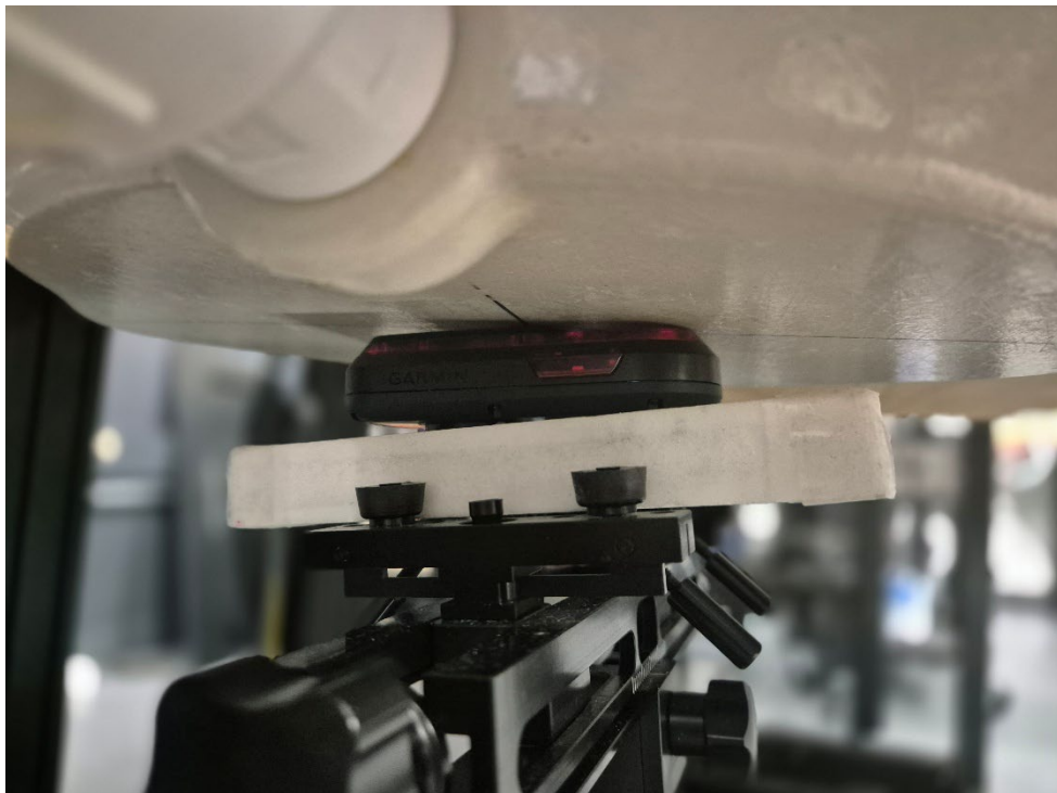
Figure 2 SAR Test Setup – Body/Extremity – Front 0mm
