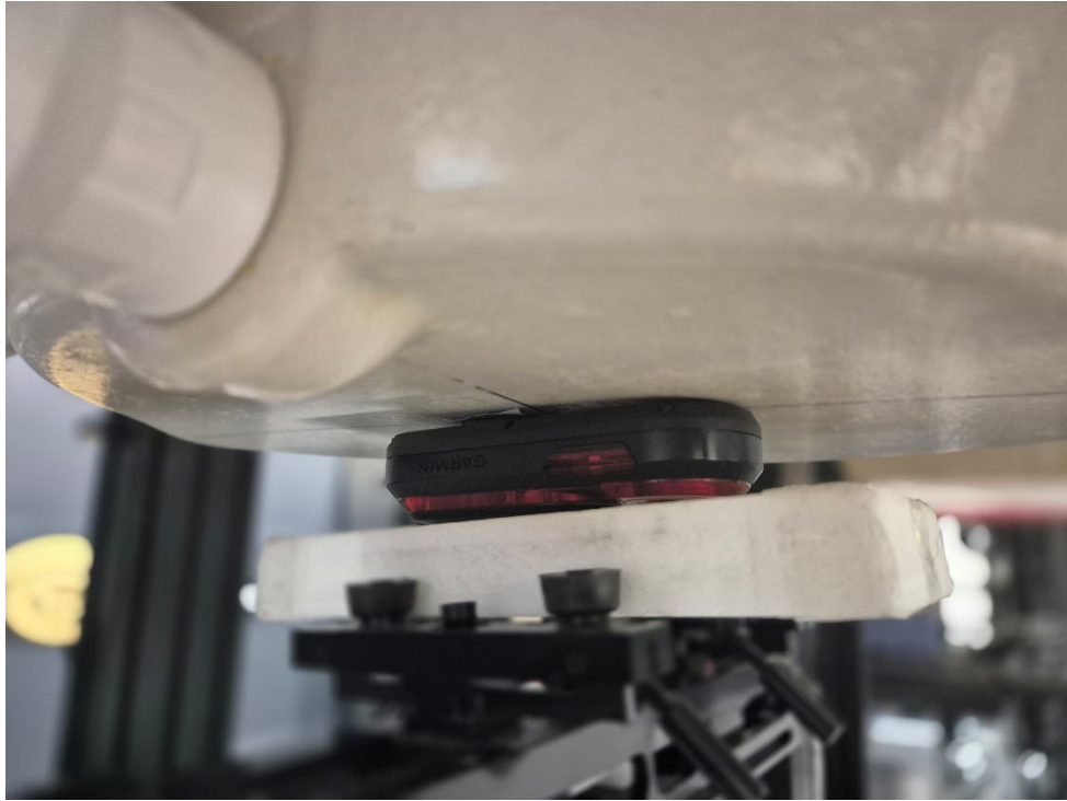
Figure 1 SAR Test Setup – Body/Extremity – Back 0mm
