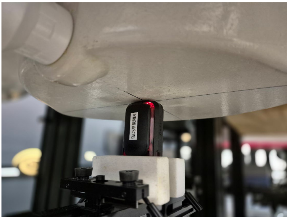
Figure 4 SAR Test Setup – Body/Extremity – Bottom 0mm
