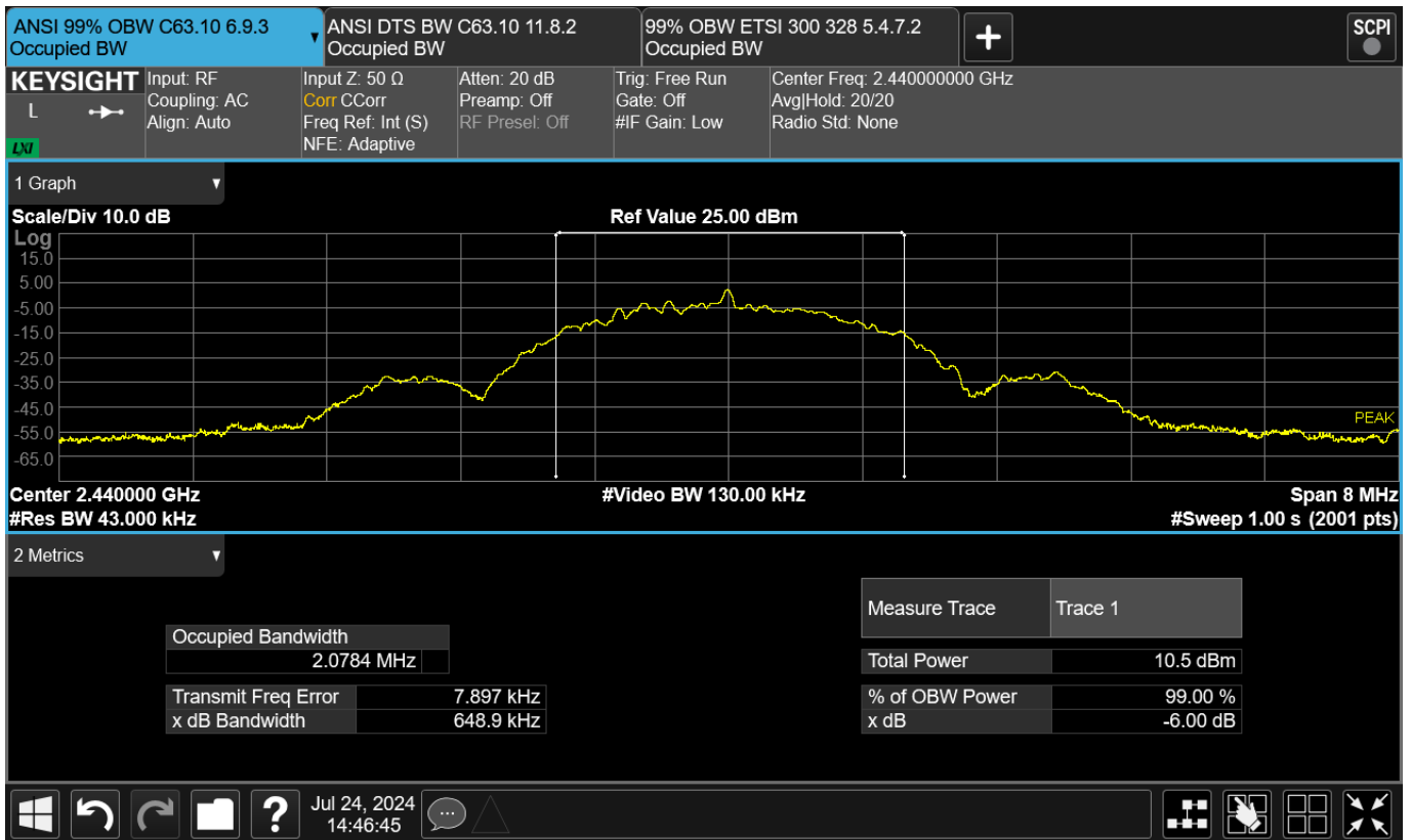
Figure TR10.3: Occupied bandwidth data for BLE 2 Mbps at mid channel (2440 MHz)
