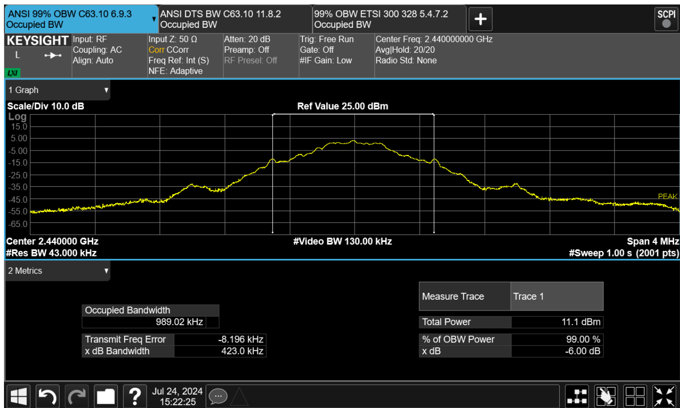
Figure TR10.4: Occupied bandwidth data for ANT at mid channel (2440 MHz)
