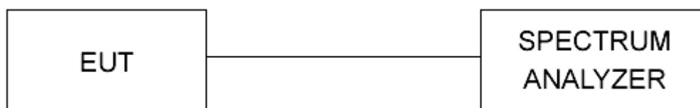
Figure 1 - Bandwidth Measurements Test Setup
