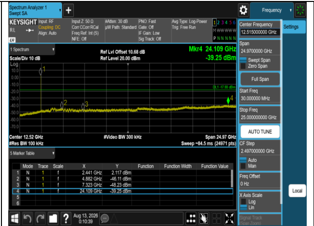
Spurious Emission GFSK 1M DH5 2441MHz
