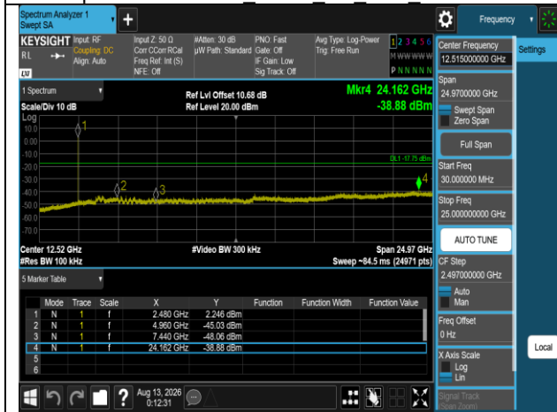
Spurious Emission GFSK 1M DH5 2480MHz
