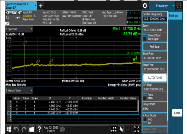
Spurious Emission 4DQPSK 2M DH5 2480MHz
