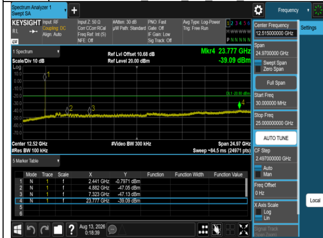
Spurious Emission 4DQPSK 2M DH5 2441MHz
