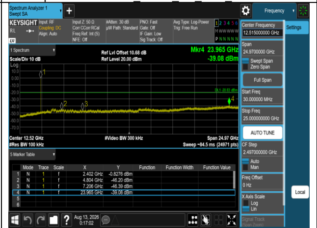
Spurious Emission 4DQPSK 2M DH5 2402MHz
