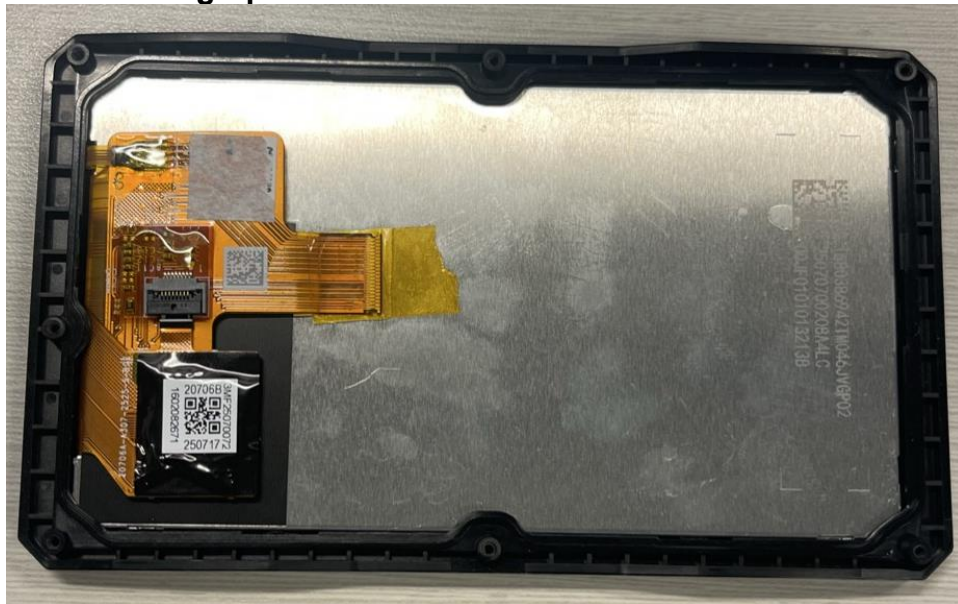
Photograph 07-7: Screen FPC with cover removed
