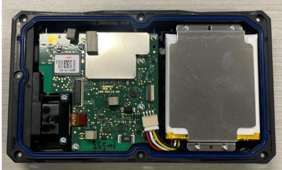
Photograph 07-1: Front side view of the main board, shield in place
