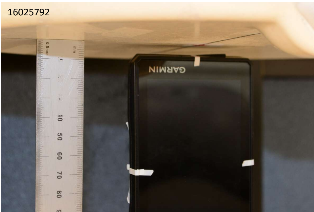
Photograph 8: Body-worn & Hotspot, Edge Left, 5 mm
