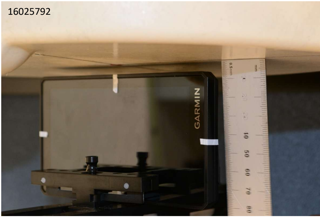
Photograph 7: Body-worn & Hotspot, Edge Bottom, 5 mm
