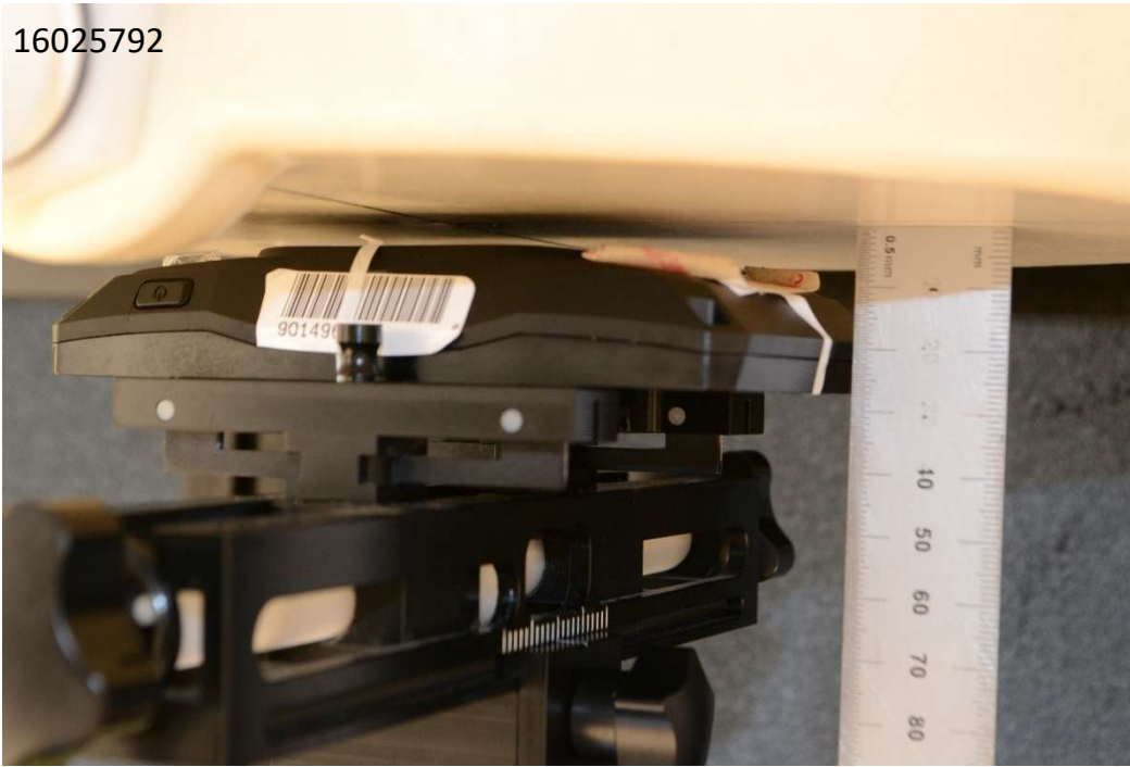
Photograph 5: Body-worn & Hotspot, Back, 5 mm
