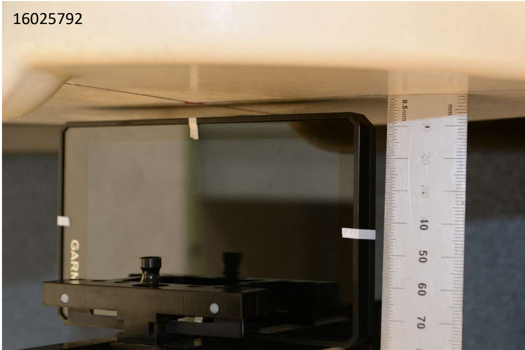
Photograph 9: Body-worn & Hotspot, Edge Top, 5 mm
