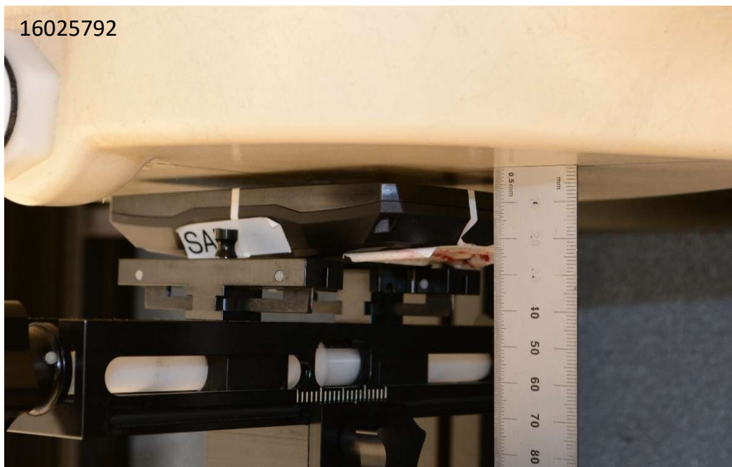
Photograph 6: Body-worn & Hotspot, Front, 5 mm
