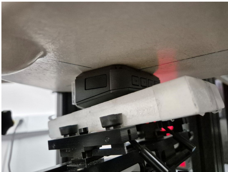
Figure 1 SAR Test Setup – Body/Extremity – Back Side 0mm
