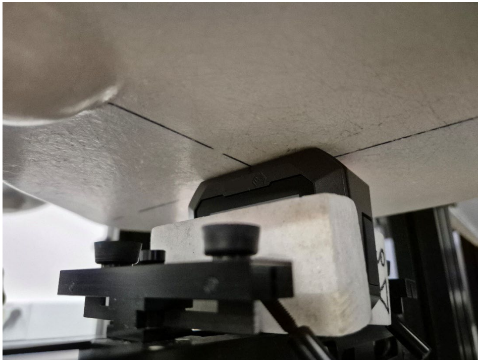
Figure 4 SAR Test Setup – Body/Extremity – Bottom Edge 0mm
