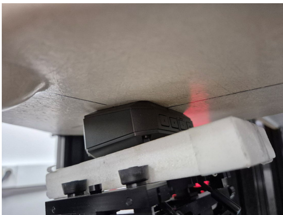
Figure 2 SAR Test Setup – Body/Extremity – Front Side 0mm
