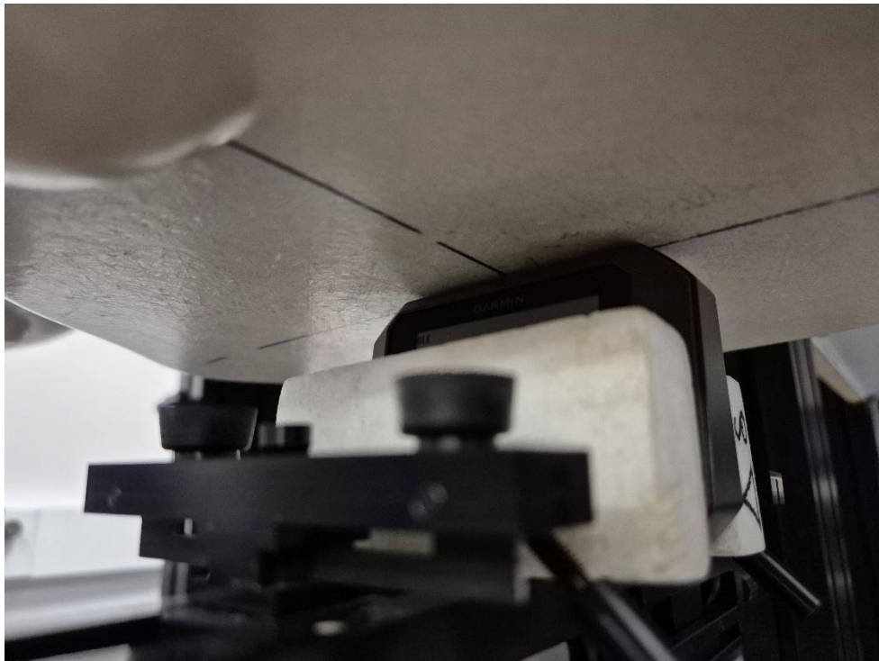
Figure 3 SAR Test Setup – Body/Extremity – Top Edge 0mm
