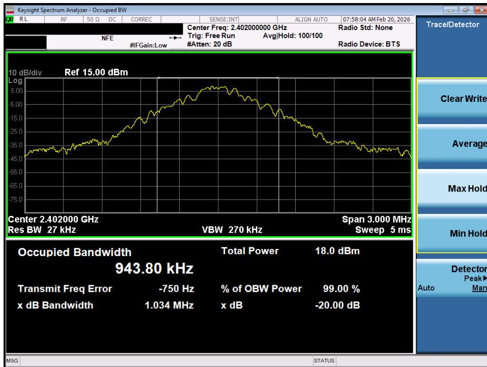
Plot 7-1. 20dB Bandwidth Plot (Bluetooth, 1Mbps – Ch. 0)
