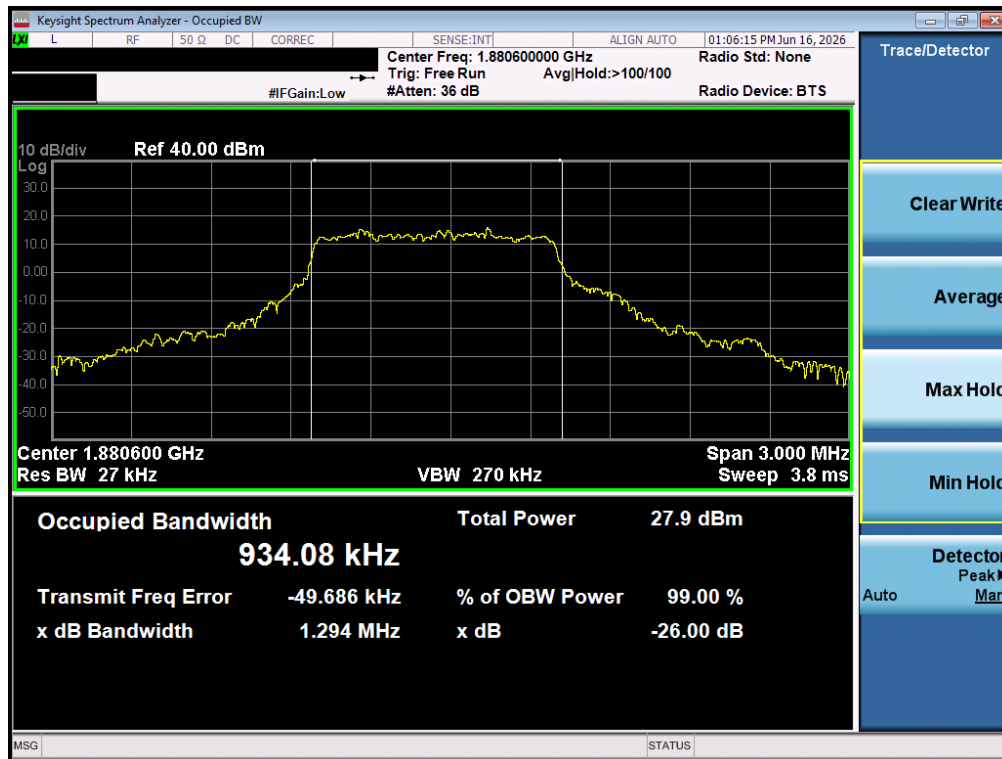
Plot 7-10. Occupied Bandwidth Plot (LTE Band 2 - 5MHz 16-QAM - Full RB - Ant1)
