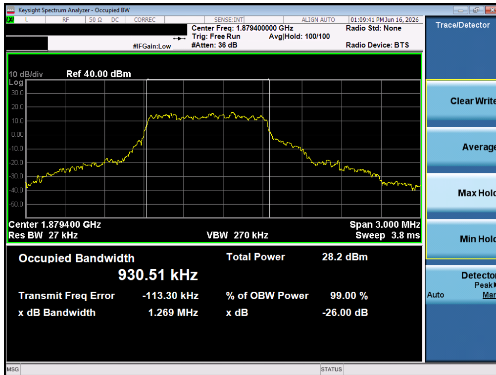
Plot 7-12. Occupied Bandwidth Plot (LTE Band 2 - 3MHz 16-QAM - Full RB - Ant1)
