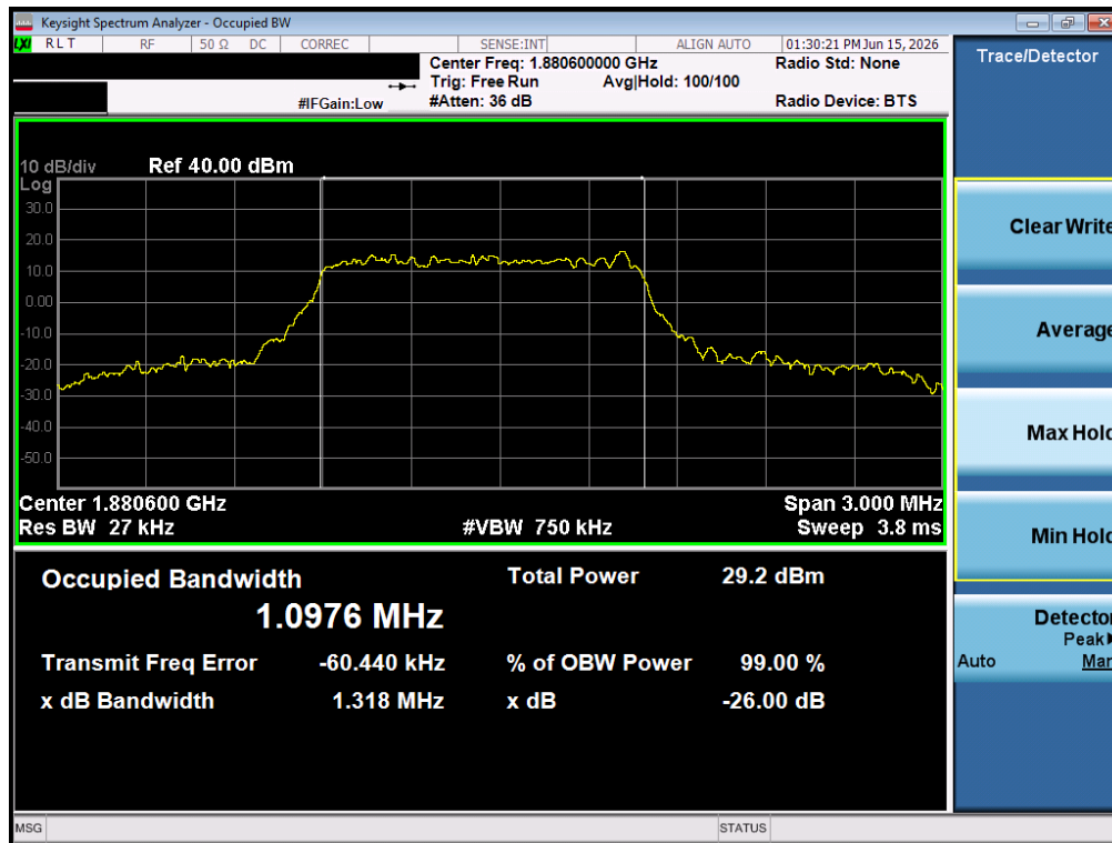
Plot 7-7. Occupied Bandwidth Plot (LTE Band 2 - 10MHz QPSK - Full RB - Ant1)
