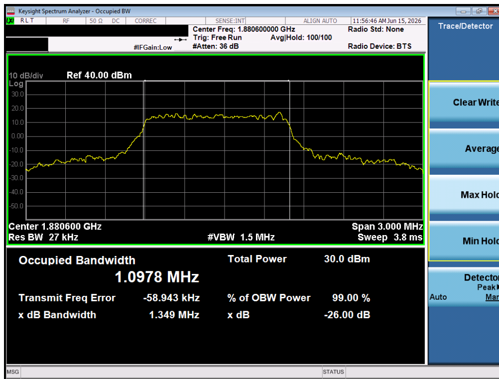
Plot 7-3. Occupied Bandwidth Plot (LTE Band 2 - 20MHz QPSK - Full RB - Ant1)
