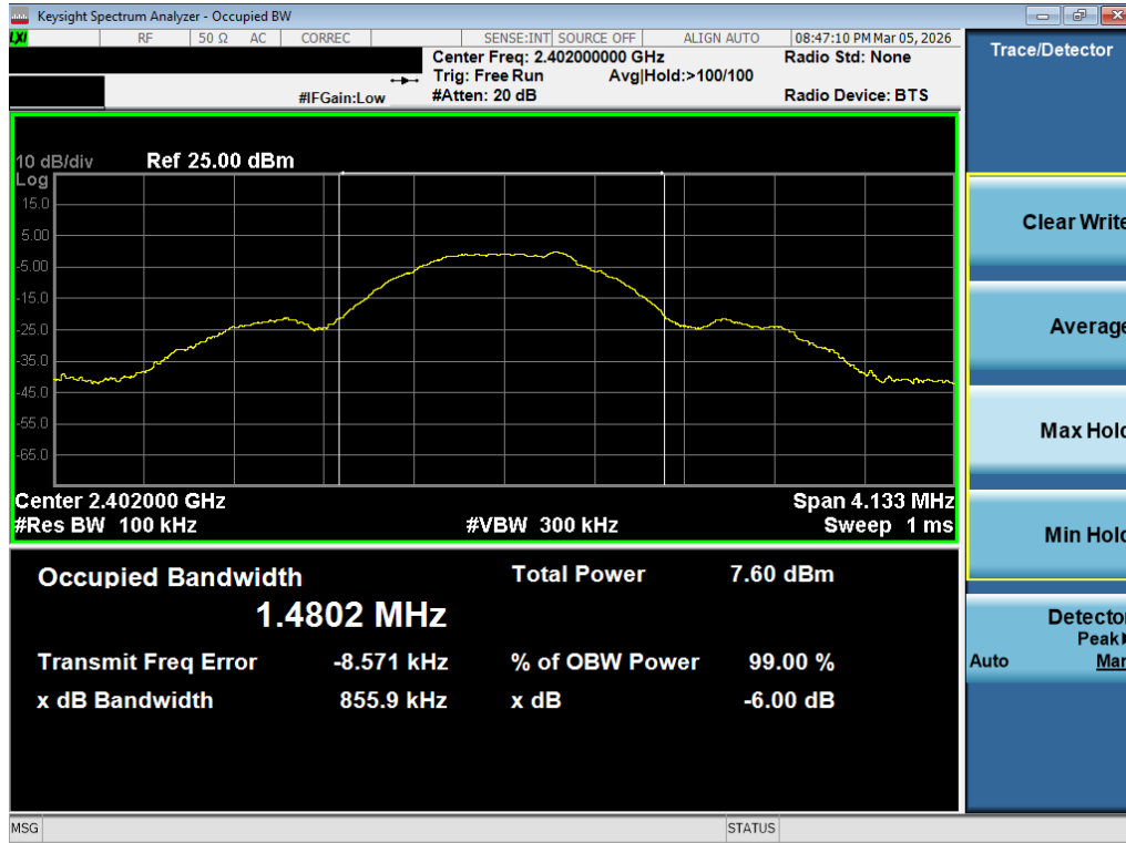
Plot 7-7. 6dB BW Plot (Bluetooth (LE), 1Mbps – Ch. 37)
