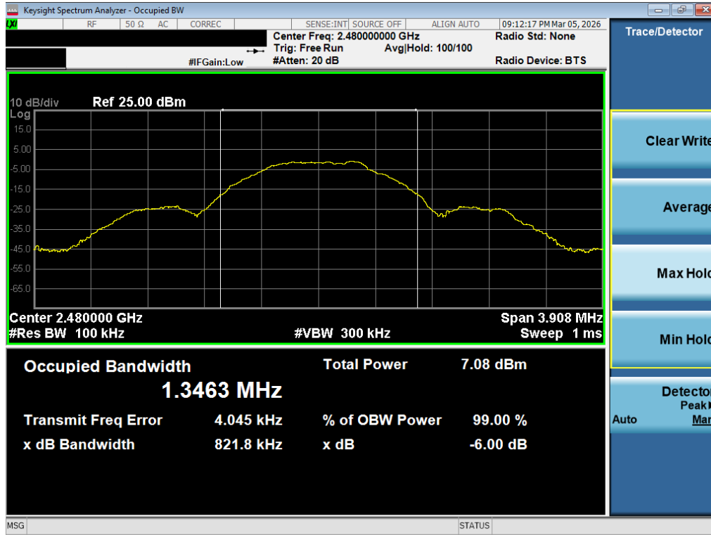
Plot 7-9. 6dB BW Plot (Bluetooth (LE), 1Mbps – Ch. 39)
