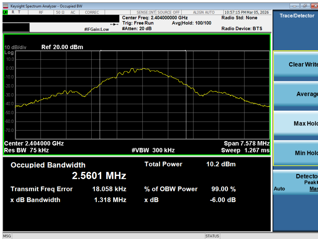
Plot 7-4. 99% OBW Plot (Bluetooth (LE), 2Mbps – Ch. 0)
