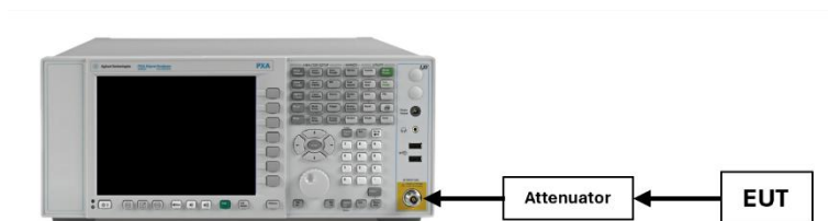
Figure 7-2. Test Instrument & Measurement Setup
