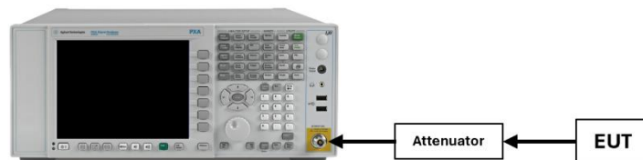
Figure 7-4. Test Instrument & Measurement Setup
