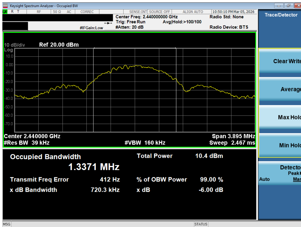
Plot 7-2. 99% OBW Plot (Bluetooth (LE), 1Mbps – Ch. 17)
