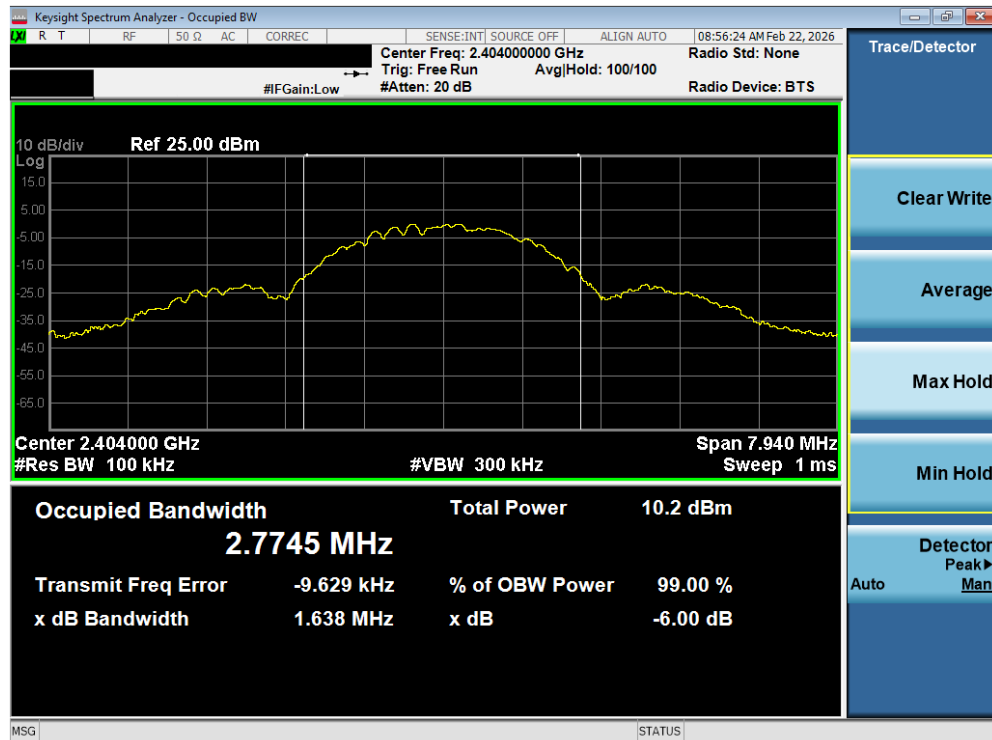
Plot 7-10. 6dB BW Plot (Bluetooth (LE), 2Mbps – Ch. 0)
