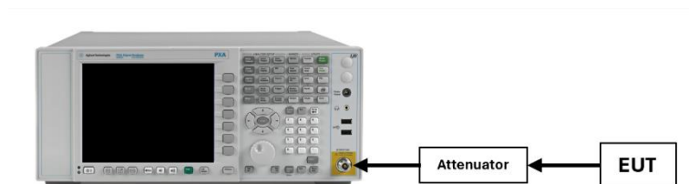
Figure 7-2. Test Instrument & Measurement Setup
