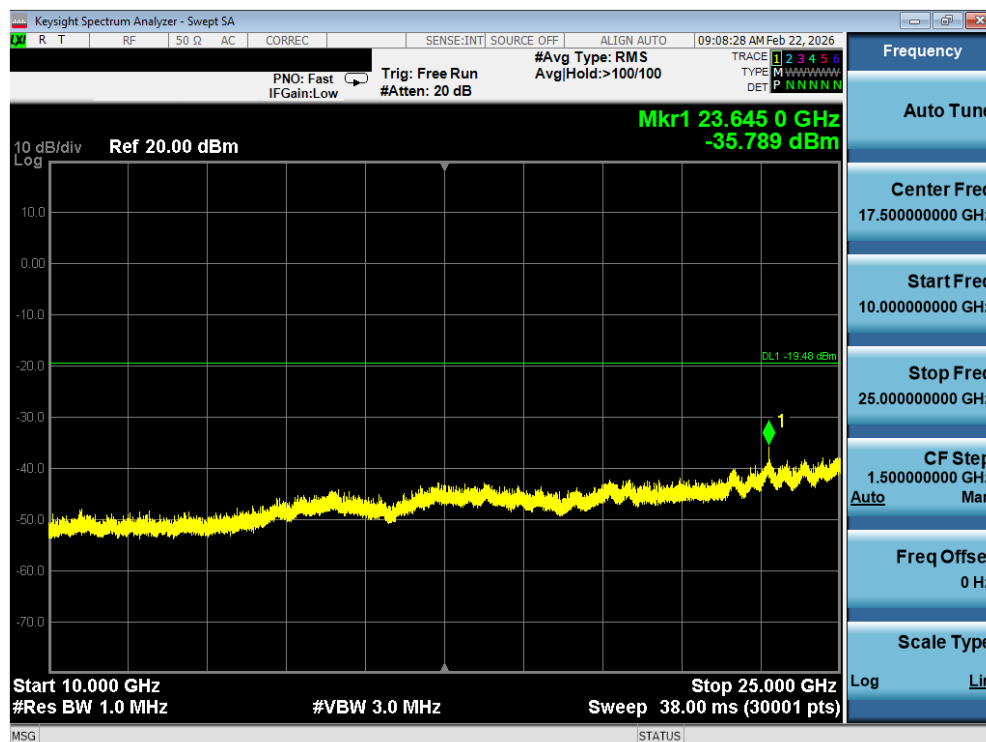
Plot 7-32. Conducted Spurious Plot (Bluetooth (LE), 1Mbps – Ch. 39)
