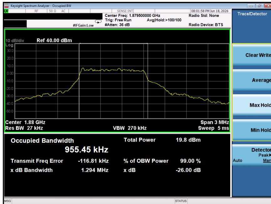
Plot 7-3. Occupied Bandwidth Plot (LTE Band 2 - 20MHz 16-QAM - Full RB)
