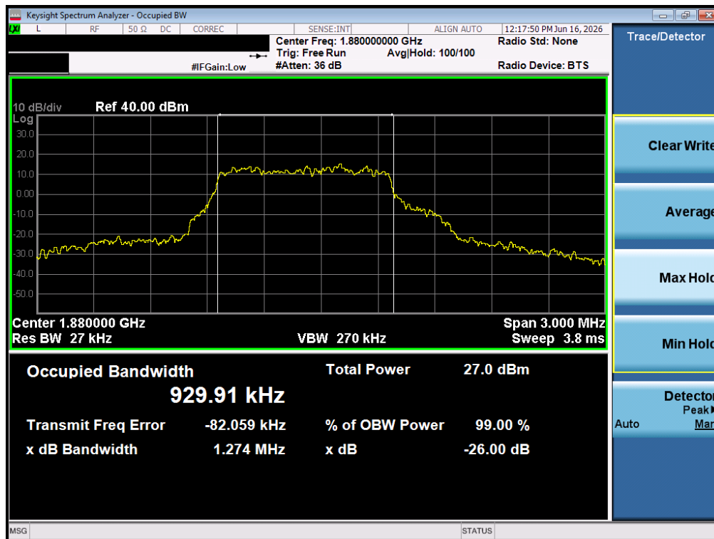
Plot 7-14. Occupied Bandwidth Plot (LTE Band 2 - 1.4MHz 16-QAM - Full RB - Ant1)
