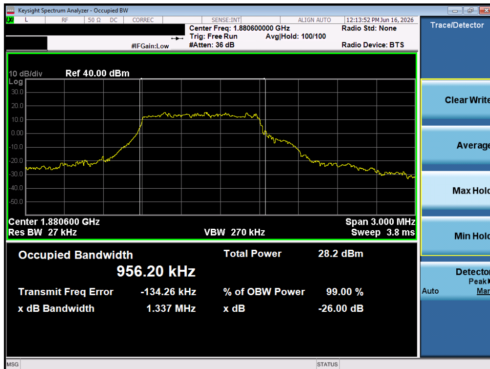
Plot 7-8. Occupied Bandwidth Plot (LTE Band 2 - 10MHz 16-QAM - Full RB - Ant1)
