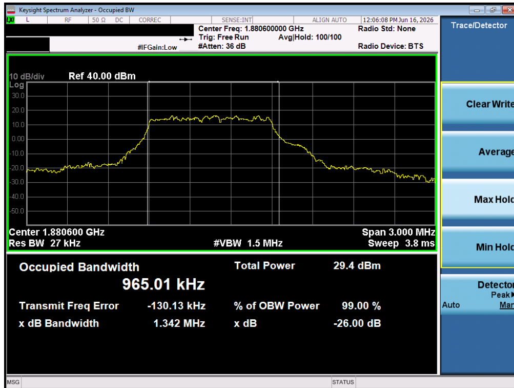
Plot 7-4. Occupied Bandwidth Plot (LTE Band 2 - 20MHz 16-QAM - Full RB - Ant1)
