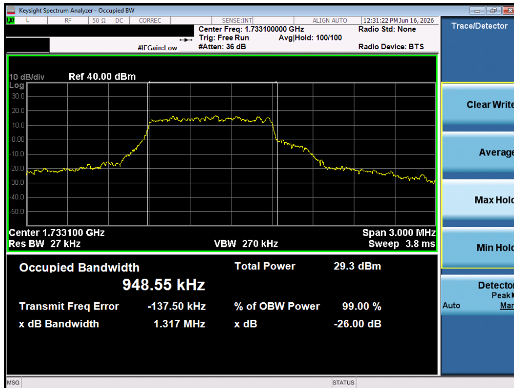
Plot 7-10. Occupied Bandwidth Plot (LTE Band 4 - 20MHz 16-QAM - Full RB - ANT1)
