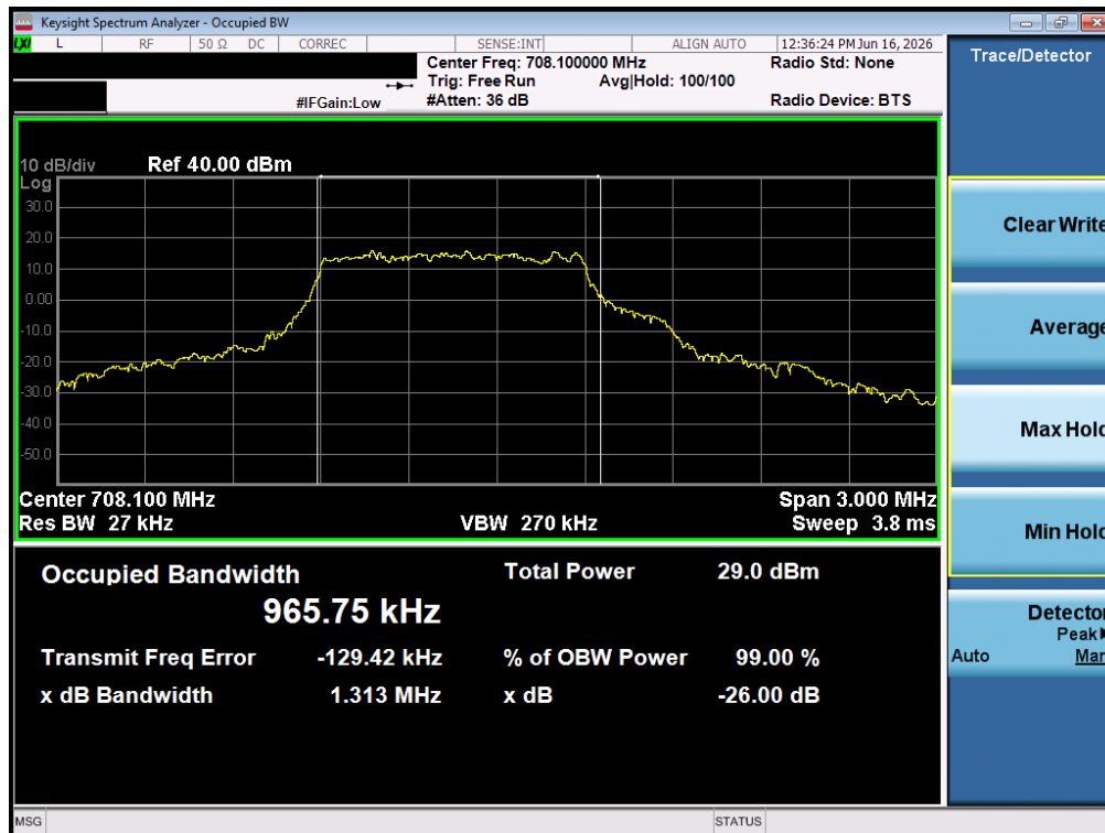
Plot 7-2. Occupied Bandwidth Plot (LTE Band 12 - 10MHz 16-QAM - Full RB – ANT1)
