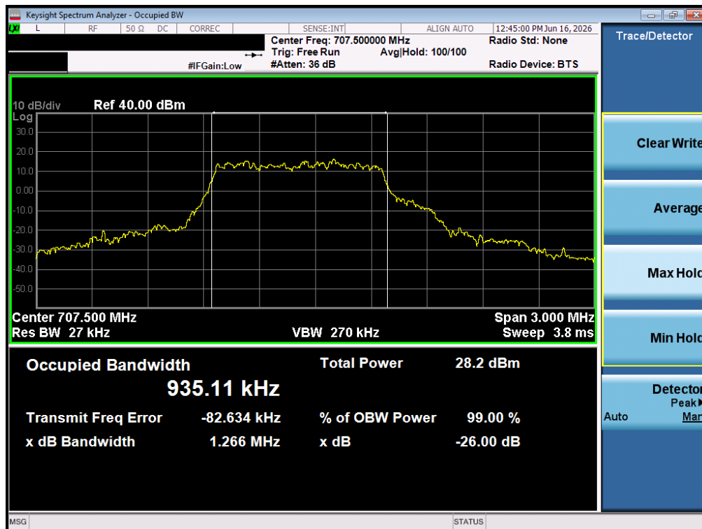
Plot 7-8. Occupied Bandwidth Plot (LTE Band 12 – 1.4MHz 16-QAM - Full RB – ANT1)
