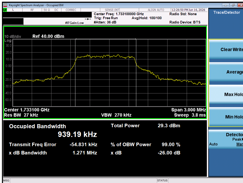
Plot 7-12. Occupied Bandwidth Plot (LTE Band 4 - 15MHz 16-QAM - Full RB - ANT1)
