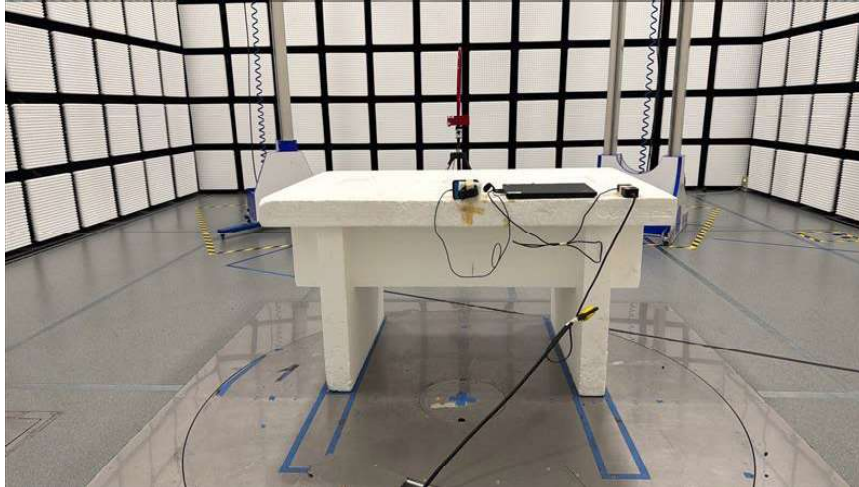
RADIATED EMISSIONS SETUP (NFC TAG ON <30MHz)
