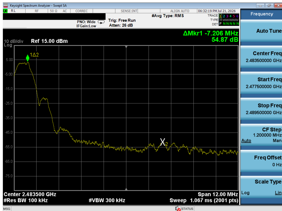
Plot 7-24. Band Edge Plot (ANT/ANT+ – Ch. 77)
