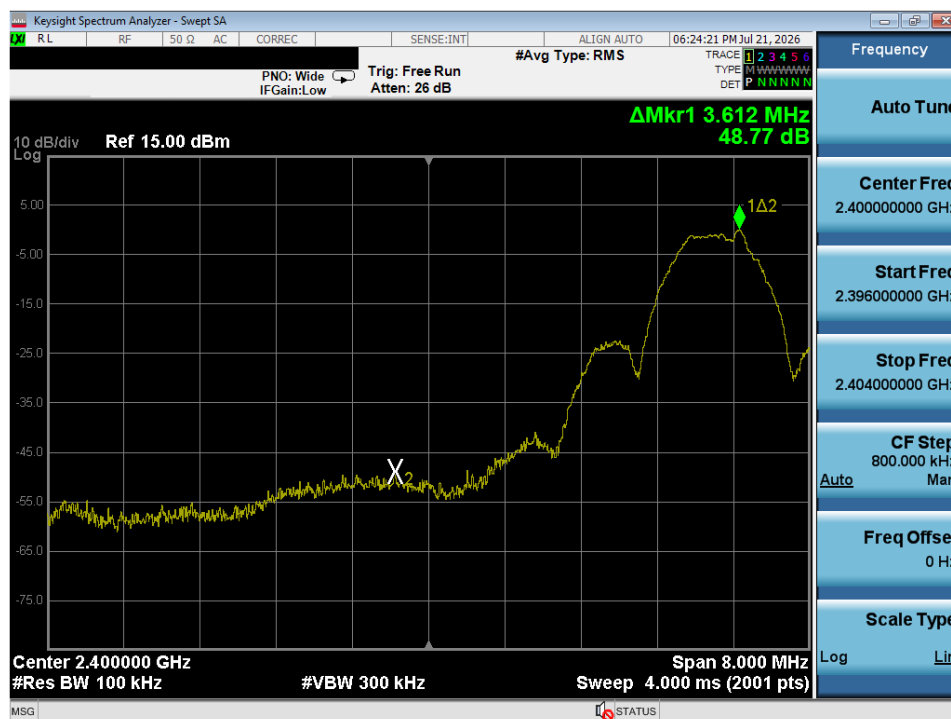
Plot 7-22. Band Edge Plot (ANT/ANT+ – Ch. 2)
