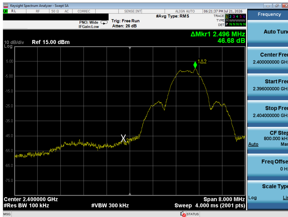
Plot 7-21. Band Edge Plot (ANT/ANT+ – Ch. 1)
