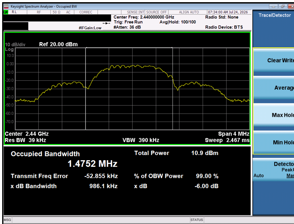
Plot 7-5. Occupied Bandwidth Plot (ANT/ANT+ – Ch. 39)
