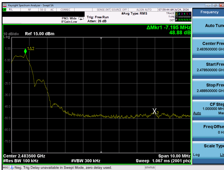
Plot 7-25. Band Edge Plot (ANT/ANT+ – Ch. 78)
