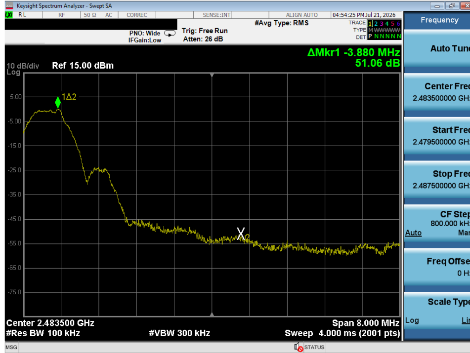
Plot 7-41. Band Edge Plot (Bluetooth (LE), 1Mbps – Ch. 39)
