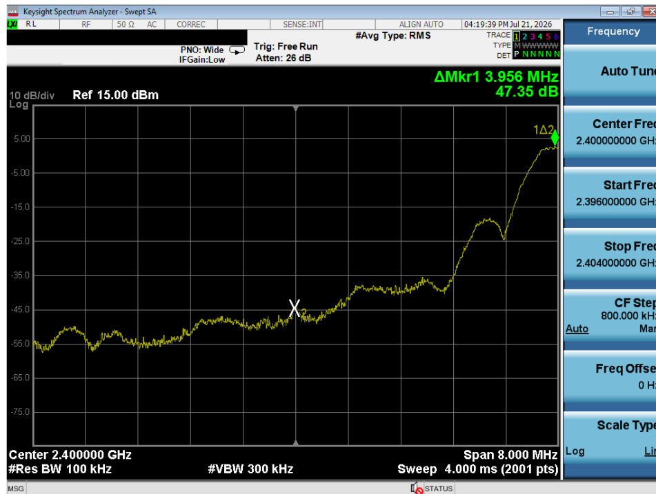
Plot 7-38. Band Edge Plot (Bluetooth (LE), 1Mbps – Ch. 37)
