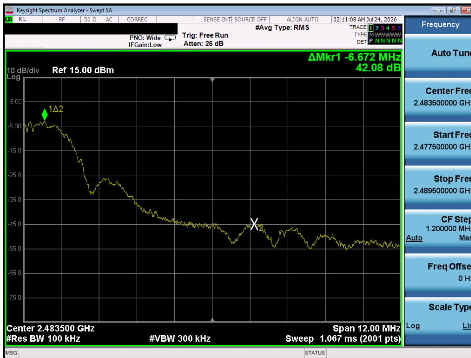
Plot 7-44. Band Edge Plot (Bluetooth (LE), 2Mbps – Ch. 36)
