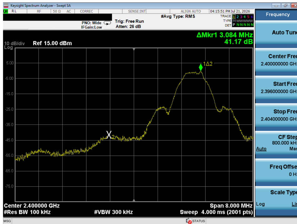
Plot 7-37. Band Edge Plot (Bluetooth (LE), 1Mbps – Ch. 37)
