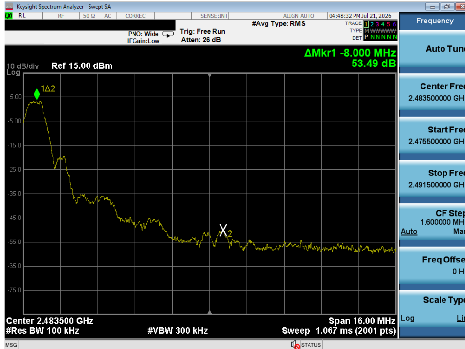
Plot 7-39. Band Edge Plot (Bluetooth (LE), 1Mbps – Ch. 35)
