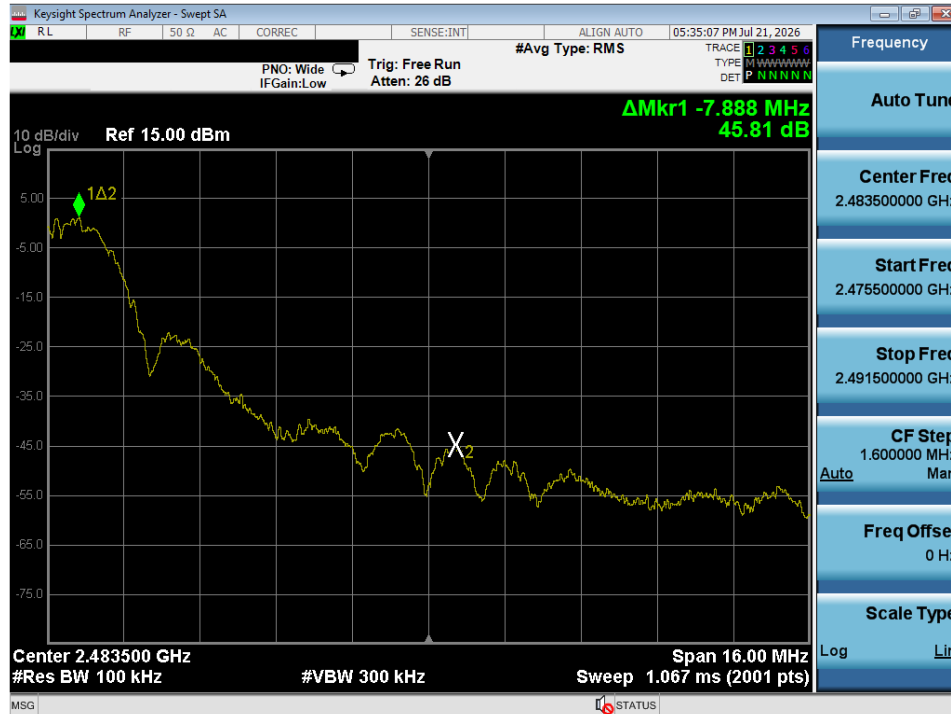
Plot 7-43. Band Edge Plot (Bluetooth (LE), 2Mbps – Ch. 35)
