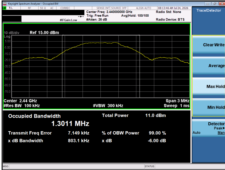
Plot 7-3. 6dB Bandwidth Plot (Bluetooth (LE), 1Mbps – Ch. 17)
