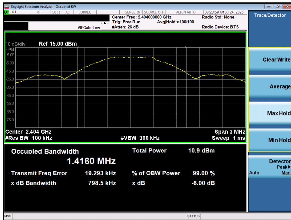
Plot 7-2. 6dB Bandwidth Plot (Bluetooth (LE), 1Mbps – Ch. 0)
