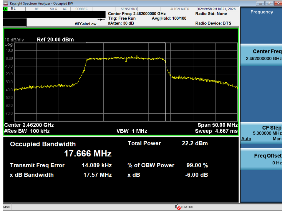
Plot 7-9. 6dB Bandwidth Plot (802.11n – Ch. 11)
