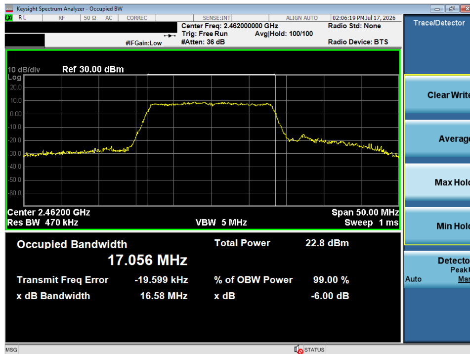
Plot 7-15. OBW Plot SISO ANT1 (802.11g – Ch. 11)
