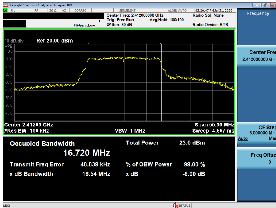
Plot 7-4. 6dB Bandwidth Plot (802.11g – Ch. 1)
