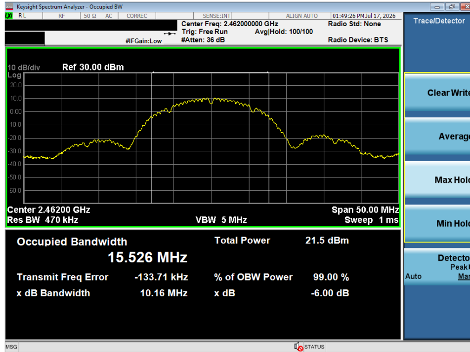
Plot 7-12. OBW Plot SISO ANT1 (802.11b – Ch. 11)
