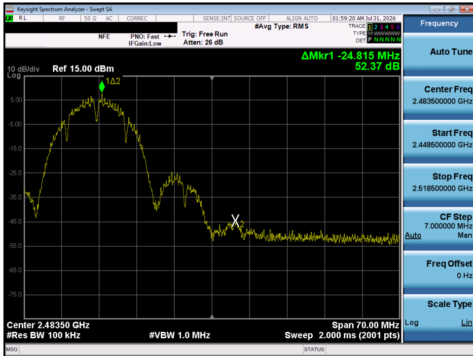
Plot 7-34. Band Edge Plot (802.11b – Ch. 11)
