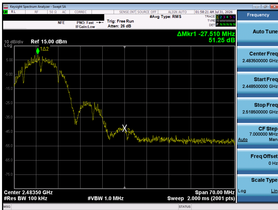
Plot 7-33. Band Edge Plot (802.11b – Ch. 10)
