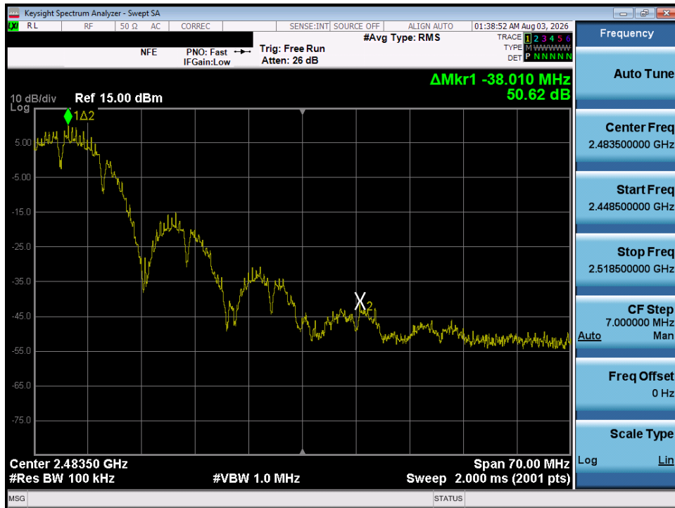
Plot 7-32. Band Edge Plot (802.11b – Ch. 9)
