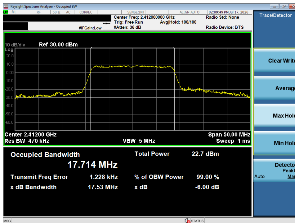
Plot 7-16. OBW Plot SISO ANT1 (802.11n- Ch. 1)
