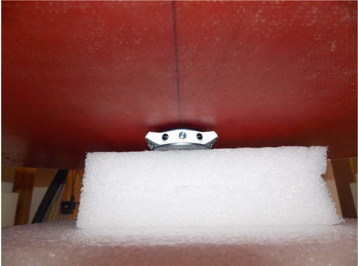
Test Position Back No Strap 0 mm Gap
