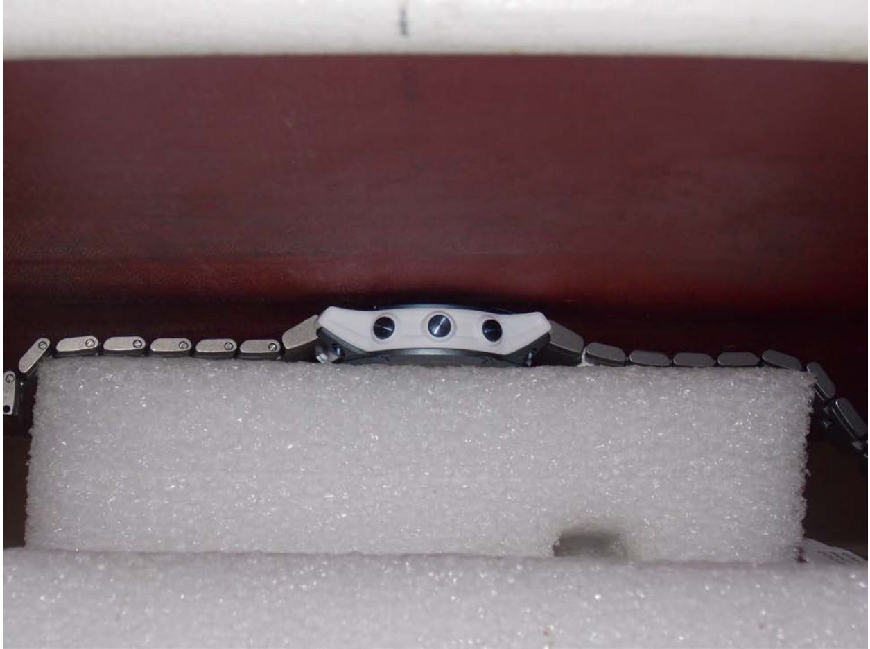
Test Position Back Metal Strap 0 mm Gap
