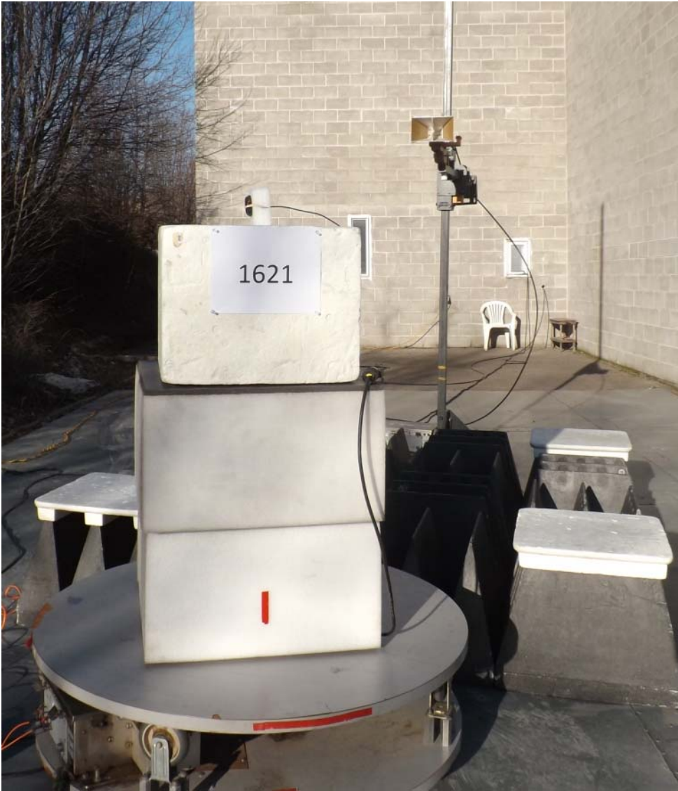
Figure E16.4 – Setup, Radiated Measurements, 1 – 18GHz
