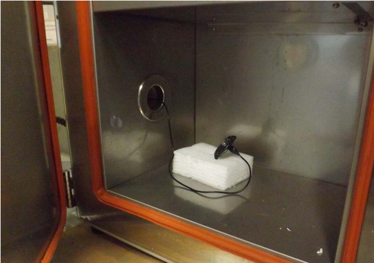
Figure E16.8 – Setup, NFC Frequency Stability Measurements
