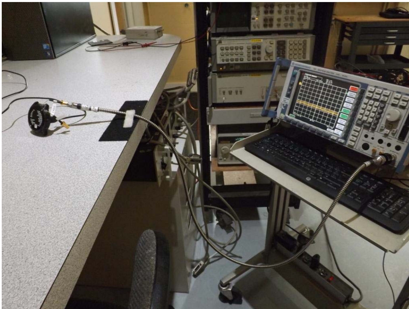
Figure E16.1 – Setup, Conducted Measurements
