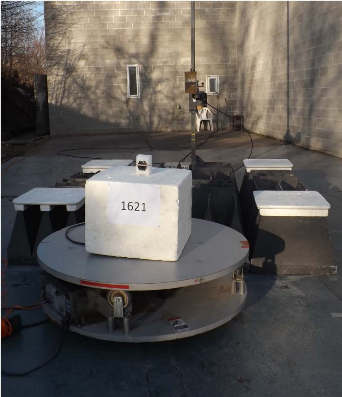
Figure E16.6 – Setup, Radiated Rx Measurements, 1 - 18GHz
