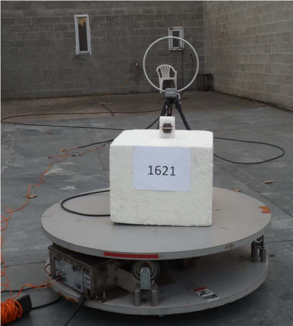
Figure E16.2 – Setup, Radiated Measurements <30MHz
