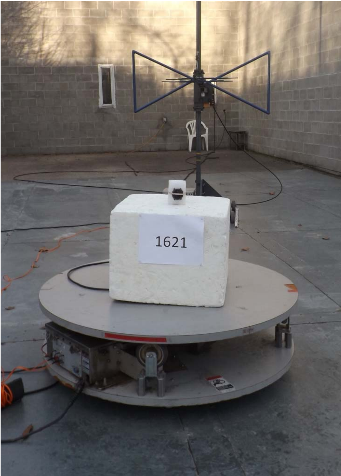
Figure E16.3 – Setup, Radiated Measurements 30 – 1000MHz
