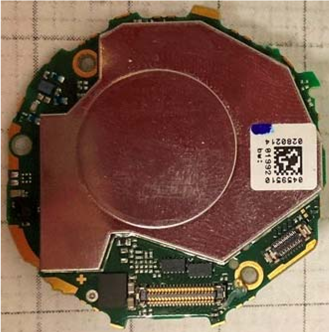
Figure E15.4 – Internal, PCB Top Side
