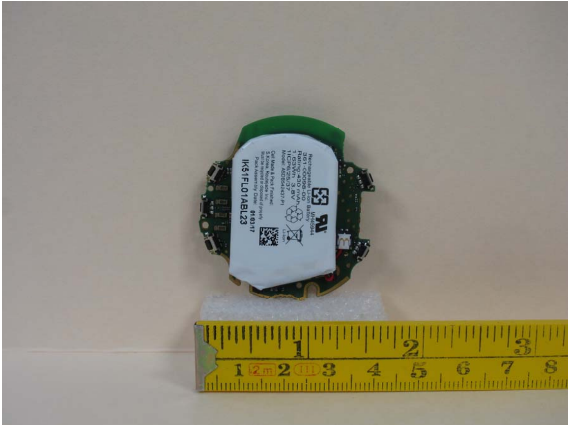
PCB Back – Battery in Place
