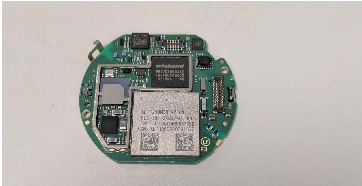
Top side of PCB [shield cover removed]
