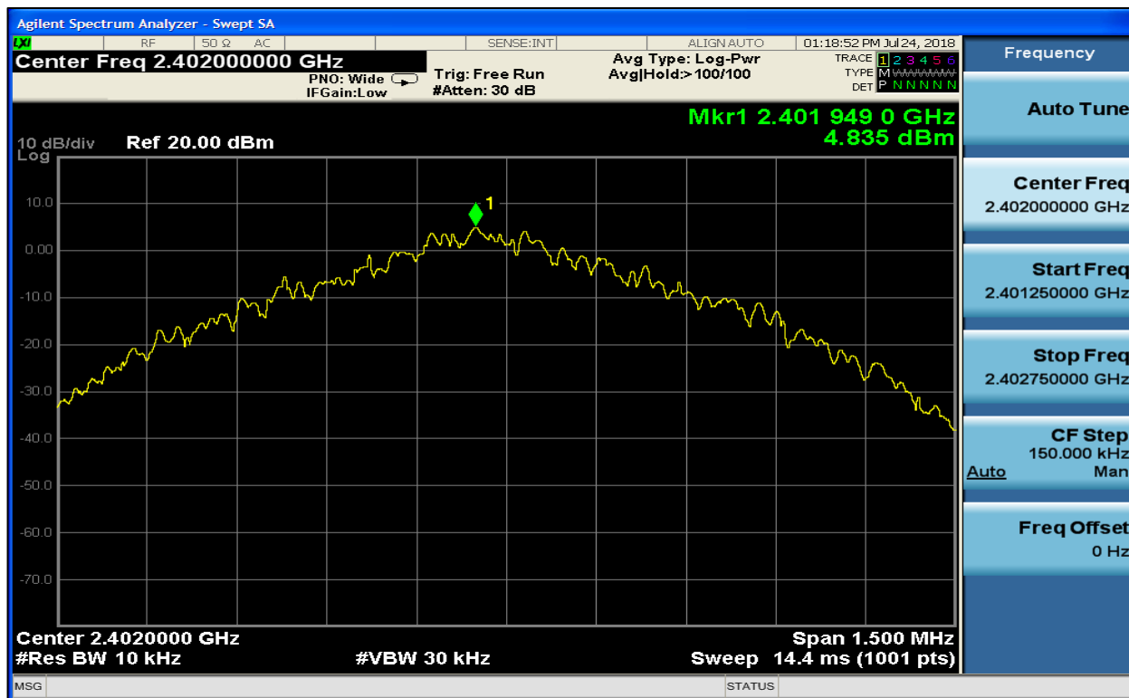
Plot 9-4: PSD – BLE – 2402 MHz
