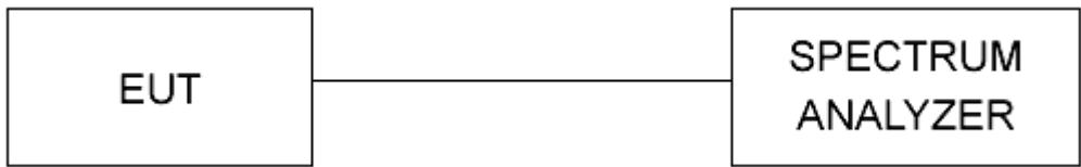
Figure 1 - Bandwidth Measurements Test Setup
