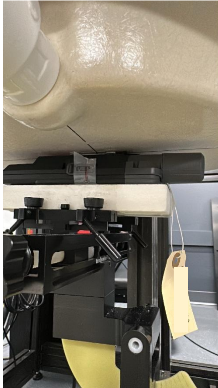
Figure A SAR Test Setup – Body/Extremity – Back 0mm
