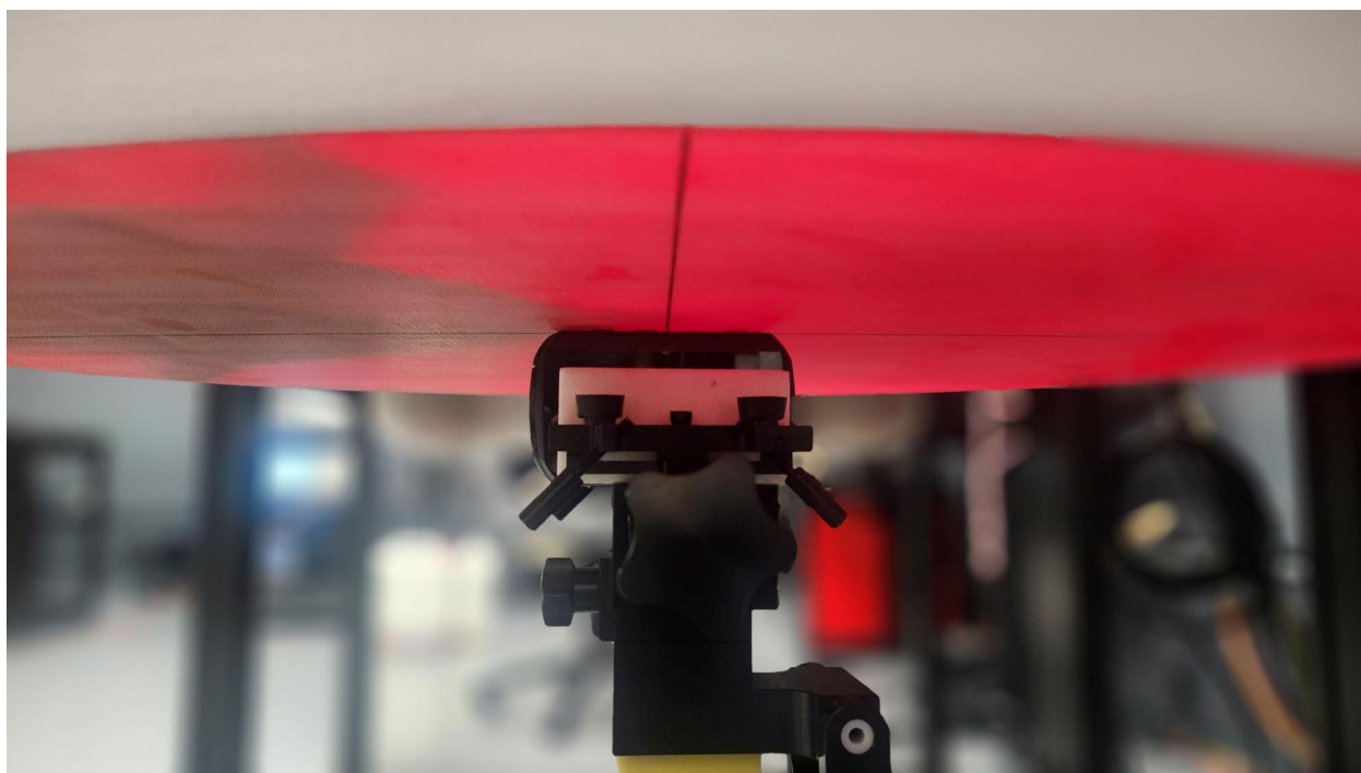
Figure M SAR Test Setup – Extremity – Left 0mm – ELI Phantom
