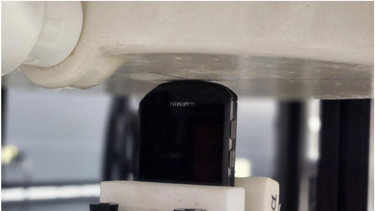
Figure E SAR Test Setup – Body/Extremity – Bottom 0mm – SAM Phantom
