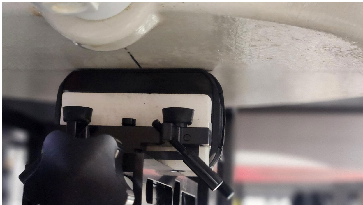
Figure F SAR Test Setup – Body/Extremity – Right 0mm – SAM Phantom
