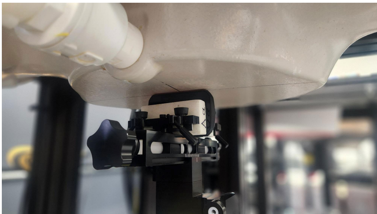
Figure G SAR Test Setup – Body/Extremity – Left 0mm – SAM Phantom
