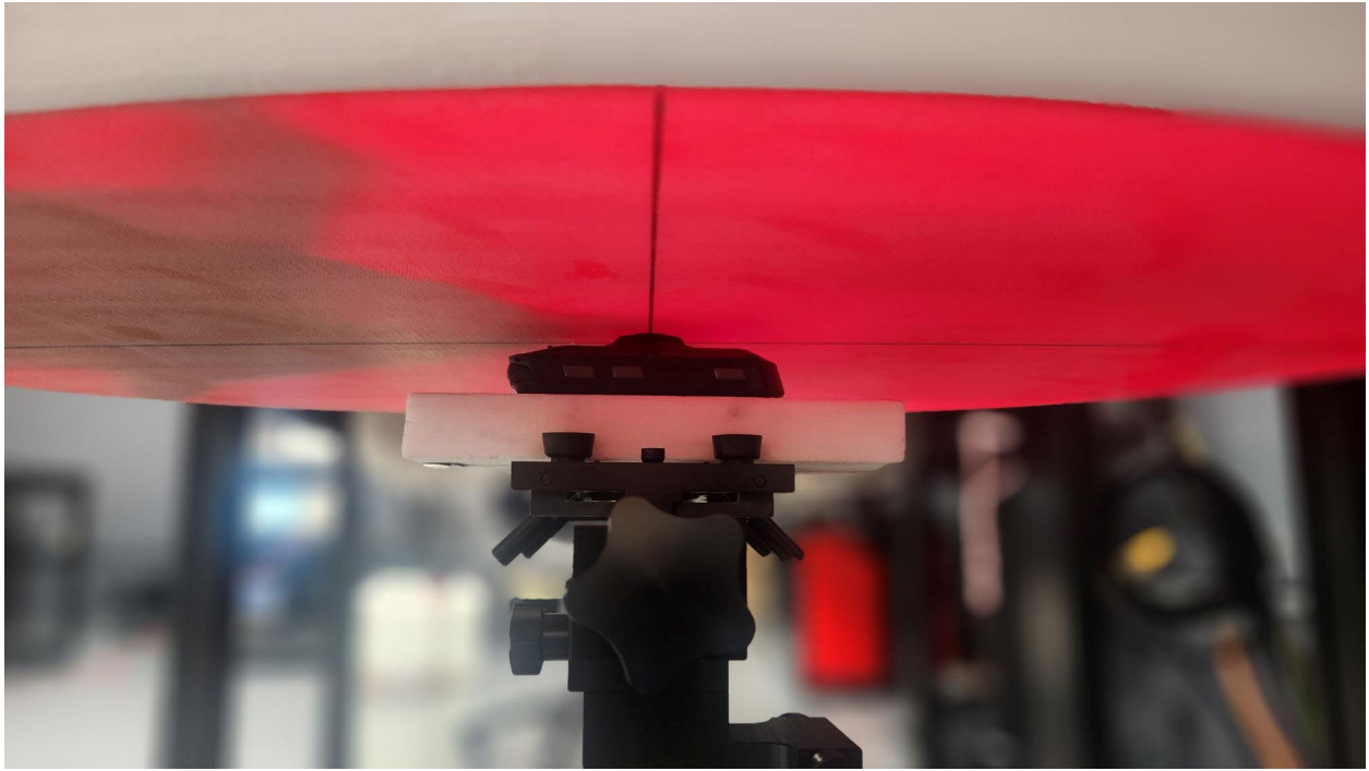
Figure H SAR Test Setup – Extremity – Back 0mm – ELI Phantom
