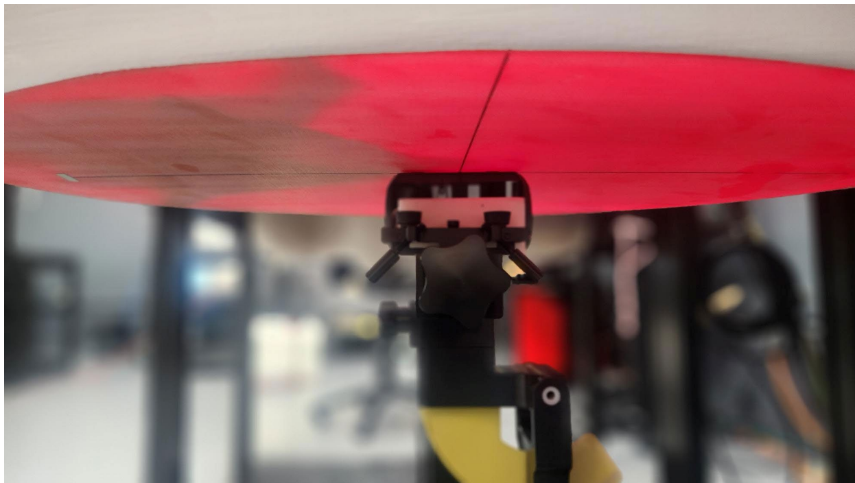
Figure L SAR Test Setup – Extremity – Right 0mm – ELI Phantom
