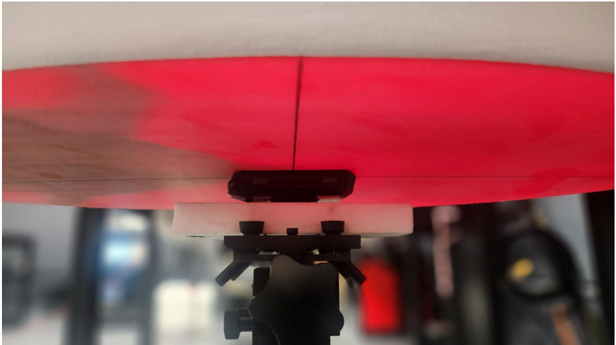
Figure I SAR Test Setup – Extremity – Front 0mm – ELI Phantom
