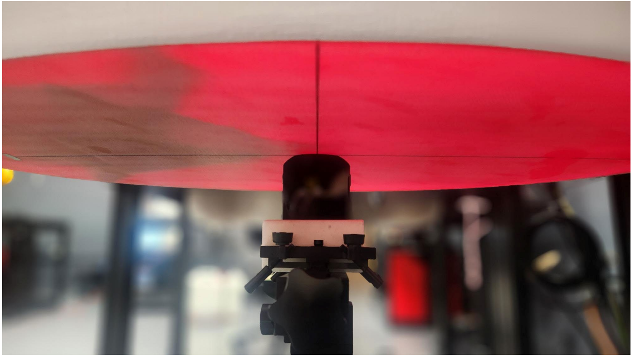
Figure J SAR Test Setup – Extremity – Top 0mm – ELI Phantom
