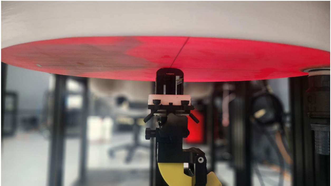
Figure K SAR Test Setup – Extremity – Bottom 0mm – ELI Phantom
