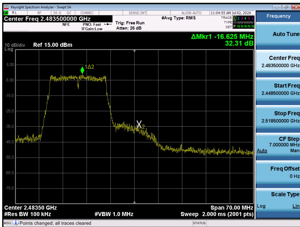
Plot 7-34. Band Edge Plot (802.11g – Ch. 12)
