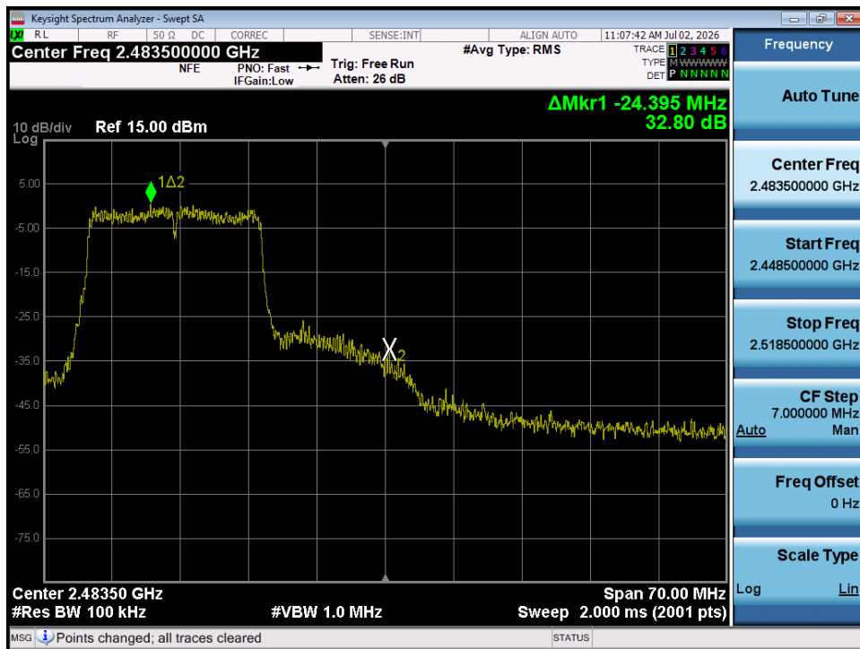
Plot 7-38. Band Edge Plot (802.11n (2.4GHz) – Ch. 11)
