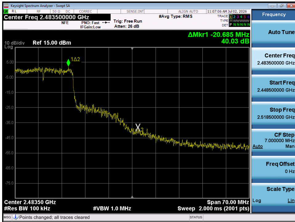
Plot 7-37. Band Edge Plot (802.11n (2.4GHz) – Ch. 10)
