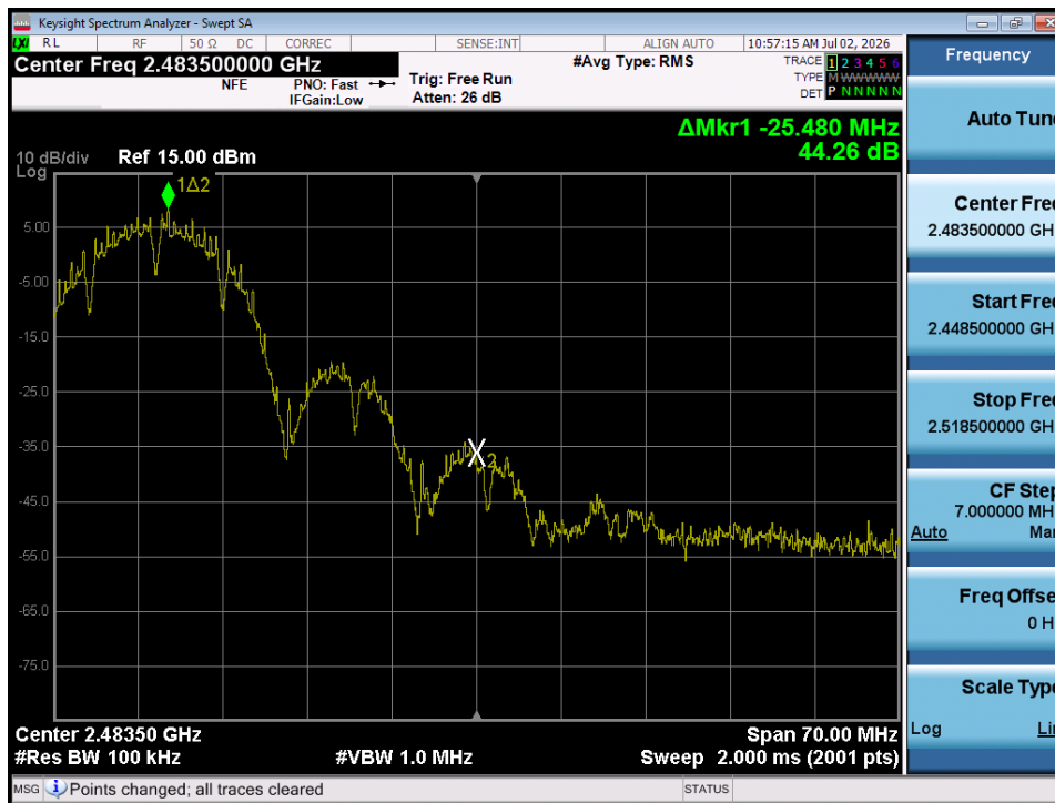
Plot 7-28. Band Edge Plot (802.11b – Ch. 10)
