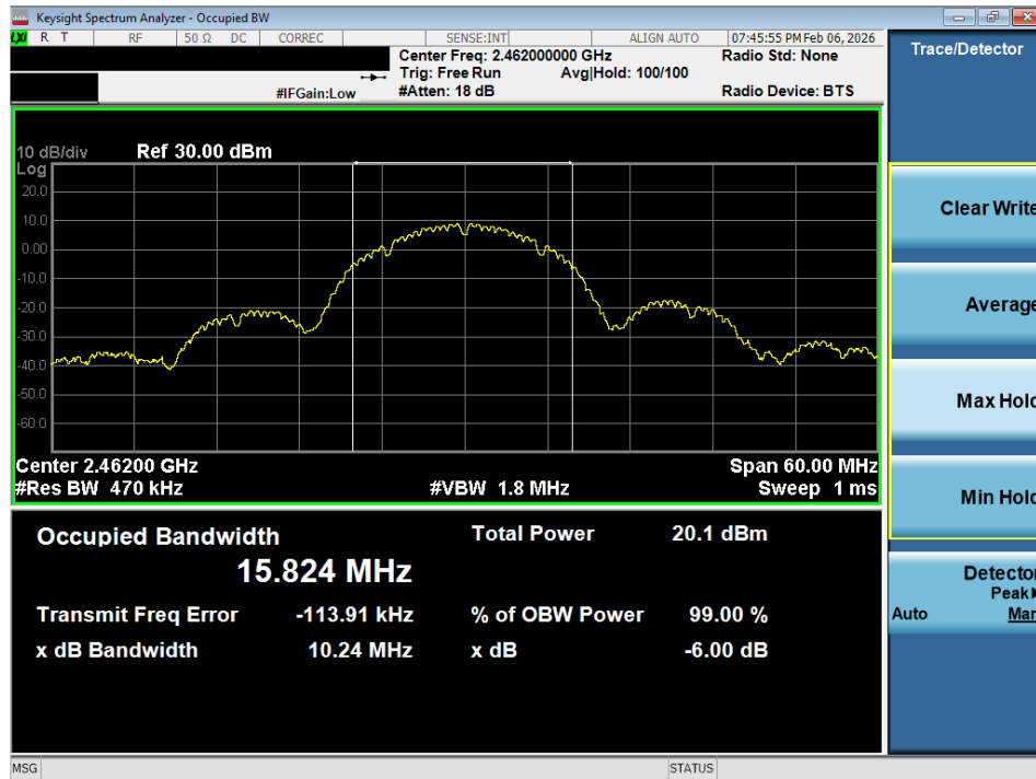
Plot 7-11 99% OBW Plot (20MHz BW 802.11b - Ch.11)
